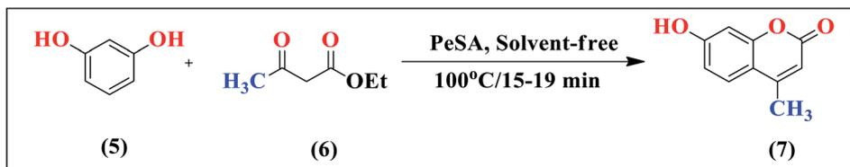
Scheme 23 Synthesis of substituted coumarins catalyzed by PeSA.
