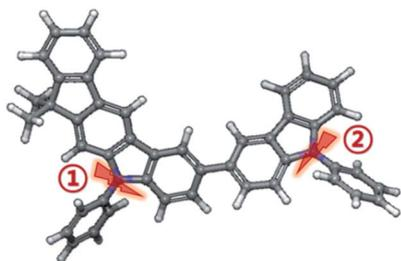
Fig. 12 Area where bond breaks in PCIC structure.
