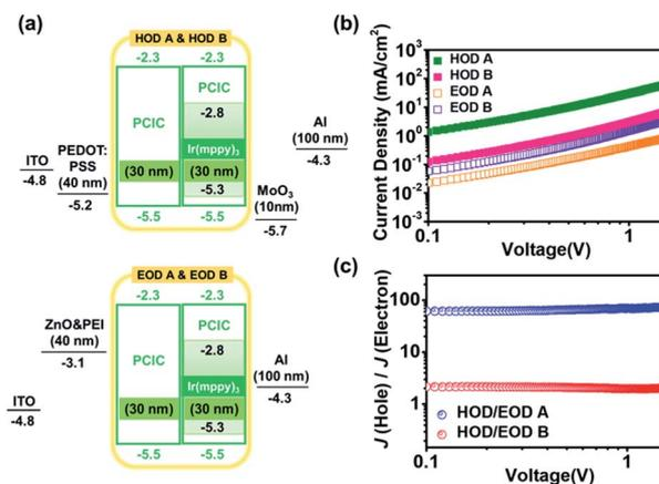
**Fig. 10** (a) HOD and EOD energy diagram consisting of pure PCIC and PCIC:Ir(mppy)<sub>3</sub> (5 mol%), (b)  $J$ - $V$  characteristics of HOD A, HOD B, EOD A and EOD B, (c) data results of  $J$  (HOD A)/ $J$  (EOD A) and  $J$  (HOD B)/ $J$  (EOD B) (device configuration with a thickness information is shown in the ESI†).
