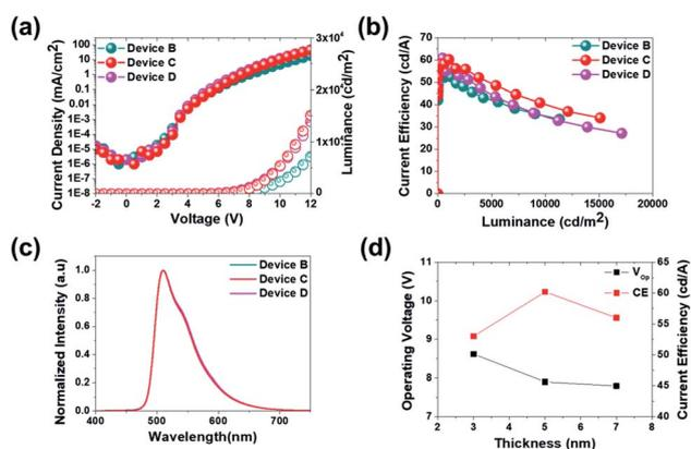
Fig. 8 (a) *J-V-L* curves, (b) current efficiency (CE) and luminance results, (c) EL spectra property, and (d) dependence of operating voltage and CE on the thickness of B-EBL at 1000 cd m<sup>-2</sup>.
