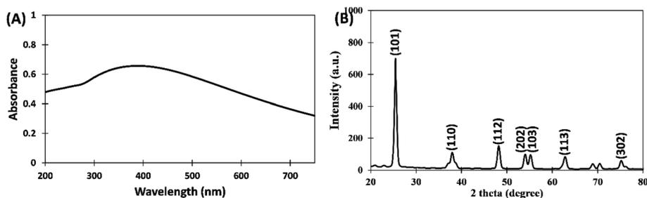
Fig. 1 (A) UV-vis absorption spectrum of titanium dioxide nanoparticles (TiO<sub>2</sub>-NPs) synthesized using aqueous extract of *Carum copticum*. (B) X-ray diffraction (XRD) pattern of TiO<sub>2</sub>-NPs.
