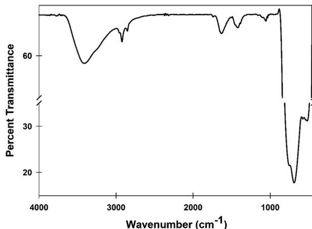
Fig. 2 Fourier-transform infrared spectroscopy (FTIR) spectrum of  $\text{TiO}_2$ -NPs. The spectrum was recorded from 4000 to 400  $\text{cm}^{-1}$  in diffuse reflectance mode at 2  $\text{cm}^{-1}$  resolution.
