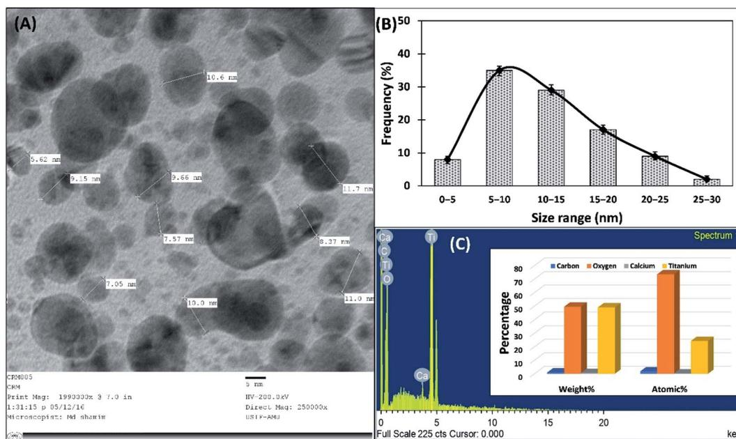
Fig. 3 (A) Transmission electron micrograph of  $\text{TiO}_2$ -NPs recorded at 25000 $\times$  magnification and 200 kV. (B) Particles size distribution of  $\text{TiO}_2$ -NPs using TEM analysis. (C) EDX spectrum and histogram of weight% and atomic% distribution (inset).
