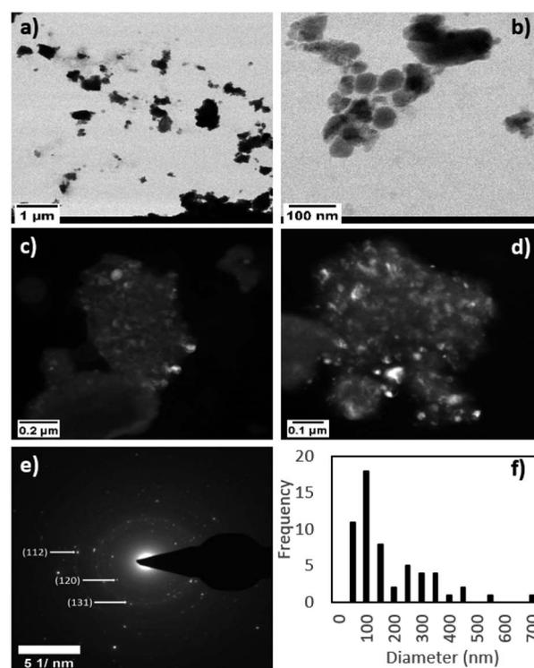
Fig. 4 Brightfield (a) and (b), and darkfield (c), and (d) STEM images at different magnifications (e) selected area electron diffraction (SAED) data and (f) grain size distribution of 180 minute-milled Co<sub>2</sub>SiO<sub>4</sub>.
