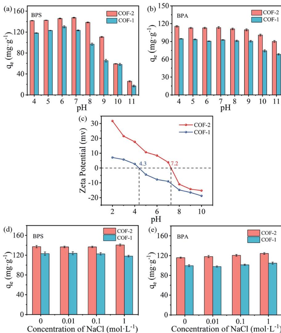
Fig. 5 (a and b) Effect of pH on BPS and BPA adsorption onto COF-1 and COF-2; (pH = 4–11,  $C_0 = 30 \text{ mg L}^{-1}$ ,  $T = 303 \text{ K}$ ,  $t = 3 \text{ h}$ ,  $m/V = 0.2 \text{ g L}^{-1}$ ); (c) zeta potential of COF-1 and COF-2; (d and e) the effect of ions strength on BPS and BPA adsorption onto COF-1 and COF-2 (NaCl concentration = 0–1  $\text{mol L}^{-1}$ ,  $C_0 = 30 \text{ mg L}^{-1}$ ,  $T = 303 \text{ K}$ ,  $t = 3 \text{ h}$ ,  $m/V = 0.2 \text{ g L}^{-1}$ ).
