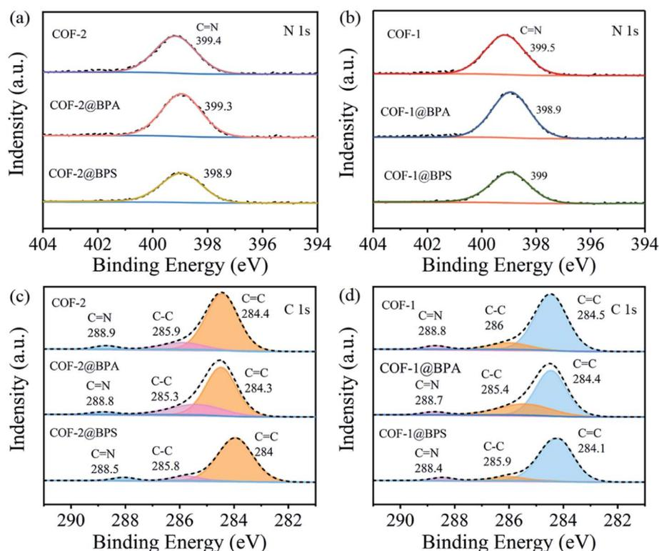
Fig. 6 (a and b) High deconvolutions of N 1s spectra of before and after adsorption of BPS and BPA onto COF-1 and COF-2; (c and d) high deconvolutions of C1s spectra of before and after adsorption of BPS and BPA onto COF-1 and COF-2.
