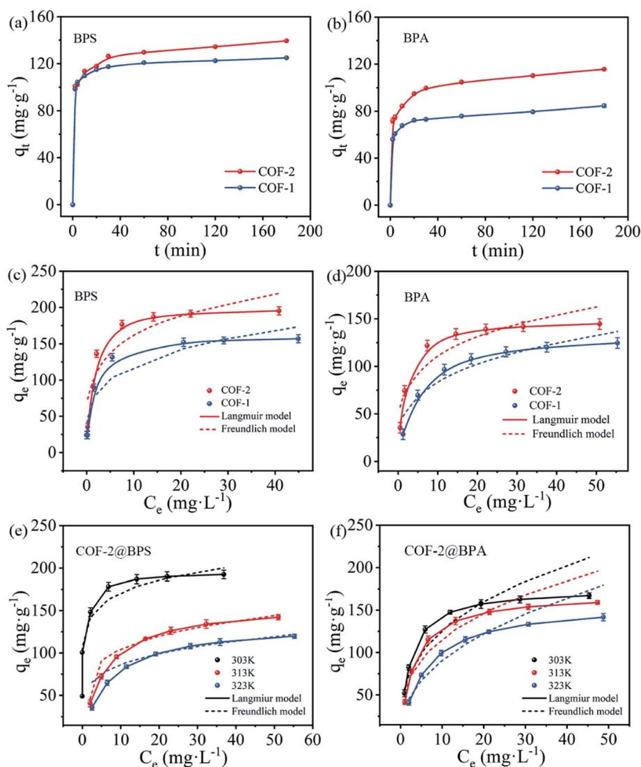
Fig. 4 (a and b) Adsorption kinetics of BPS and BPA onto COF-1 and COF-2 ( $C_0 = 30 \text{ mg L}^{-1}$ ,  $T = 303 \text{ K}$ ,  $t = 3 \text{ h}$ ,  $m/V = 0.2 \text{ g L}^{-1}$ ); (c and d) adsorption isotherm of BPS and BPA onto COF-1 and COF-2 at 303 K; (e and f) adsorption isotherms of BPS and BPA onto COF-2 at different temperatures ( $C_0 = 10\text{--}80 \text{ mg L}^{-1}$ ,  $T = 303\text{--}323 \text{ K}$ ,  $t = 24 \text{ h}$ ,  $m/V = 0.2 \text{ g L}^{-1}$ ).
