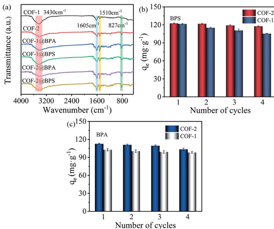
Fig. 7 (a) FT-IR spectra of before and after adsorption of BPS and BPA onto COF-1 and COF-2; (b and c) regeneration test of COF-1 and COF-2 for the adsorption of BPS and BPA (adsorption:  $C_0 = 30 \text{ mg L}^{-1}$ ,  $T = 303 \text{ K}$ ,  $t = 3 \text{ h}$ ,  $m/V = 0.2 \text{ g L}^{-1}$ ; desorption with methanol,  $t = 1 \text{ h}$ ,  $V = 40 \text{ ml}$ ).
