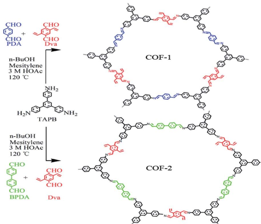
Scheme 1 The synthesis process of COF-1 and COF-2.
