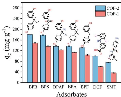
Fig. 3 Adsorption capacities of different types of pharmaceuticals onto COF-1 and COF-2 (in each case  $C_0 = 50 \text{ mg L}^{-1}$ ,  $T = 303 \text{ K}$ ,  $t = 3 \text{ h}$ ,  $m/V = 0.2 \text{ g L}^{-1}$ ).
