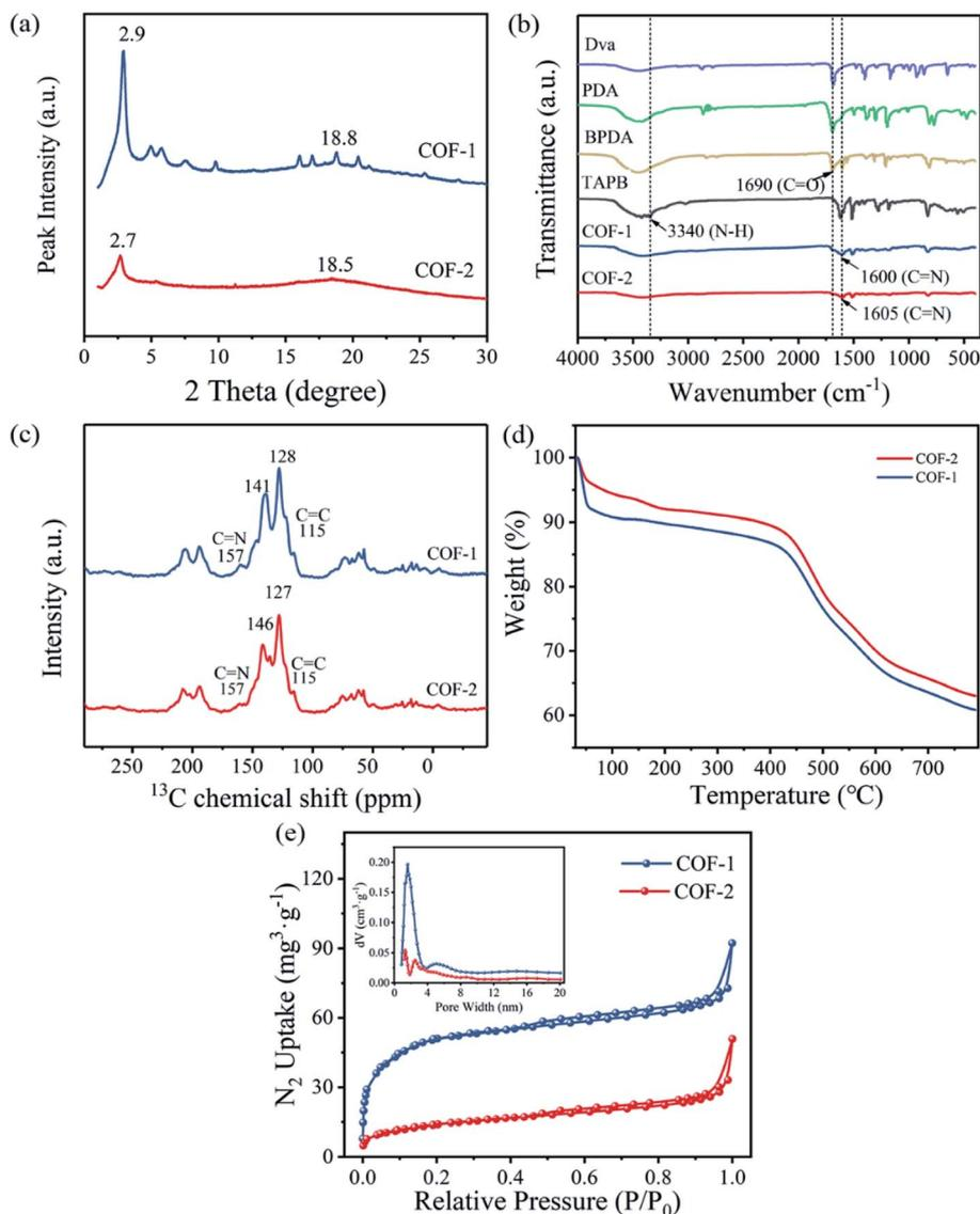
Fig. 2 (a) XRD patterns of COF-1 and COF-2; (b) FT-IR spectrum of COF-1 and COF-2; (c)  $^{13}\text{C}$  NMR spectra of COF-1 and COF-2; (d) TGA curves of COF-1 and COF-2; (e)  $\text{N}_2$  adsorption-desorption isotherm, inset: pore-size distribution of COF-1 and COF-2.
