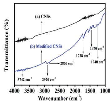
Fig. 3 FTIR spectra of (a) unmodified CNSs and (b) modified CNSs.
