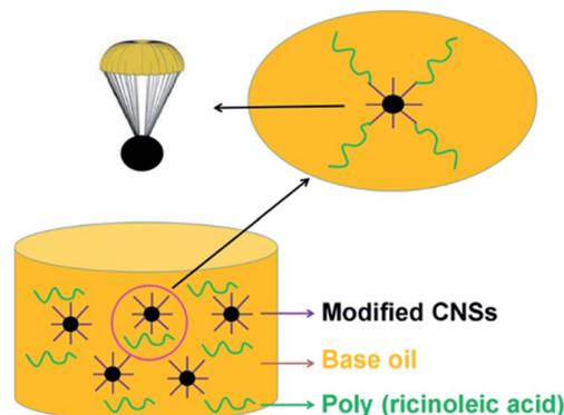
Fig. 12 Mechanism of modified CNS dispersion stability behaviors.
