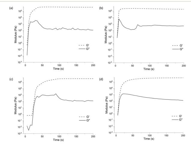
Fig. 4 Time-resolved rheology gelation curves over 200 seconds shown by G' and G'' for elastomers derived from PDMS **1b** and the (a) ethyl **2**, (b) propyl **3**, (c) n-butyl **4**, and (d) s-butyl **6** alkoxysilane (also see entries 6–10, Table 1). Note the omitted data as per Table 1.
