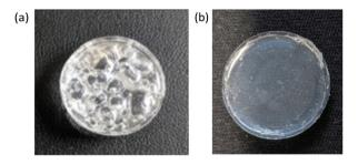
Fig. 1 Digital photographs of bulk samples of PDMS-based polymer networks illustrating the further reduction of foaming upon optimisation of the reaction conditions. Samples were prepared by reacting hydrideterminated PDMS 1a with tetra-n-butoxysilane 4 and: (a)  $5 \times 10^{-4}$  mmol  $B(C_6F_5)_3$  and (b)  $2 \times 10^{-4}$  mmol  $B(C_6F_5)_3$ .
