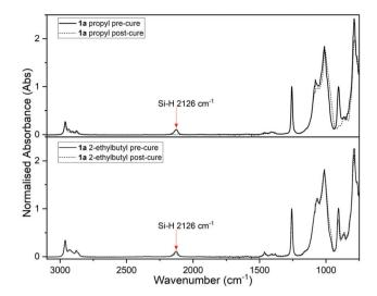
**Fig. 2** Absorbance normalised 30° grazing angle FTIR spectra for (top) PDMS system **1a** propyl **3** pre- and post-cure measurements, Si–H peak at 2126 cm<sup>-1</sup> disappears from pre- to post-cure measurements, and (bottom) PDMS system **1a** 2-ethylbutyl **5** pre- and post-cure measurements, Si–H peak found at 2126 cm<sup>-1</sup> decreases from pre- to post-cure measurements.
