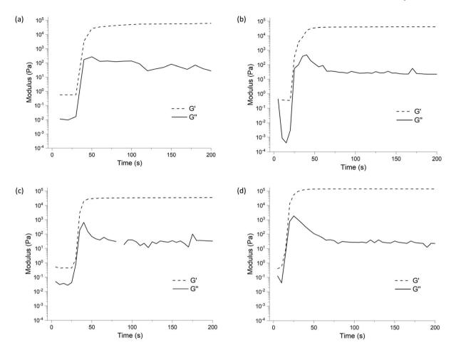
Fig. 3 Time-resolved rheology gelation curves over 200 seconds shown by G' and G'' for elastomers derived from PDMS  $\mathbf{1a}$  and the (a) ethyl  $\mathbf{2}$  note differing transition to plateau by gradual increase in modulus, (b) propyl  $\mathbf{3}$ , (c) n-butyl  $\mathbf{4}$ , and (d) s-butyl  $\mathbf{6}$  alkoxysilane (also see entries  $\mathbf{1}$ - $\mathbf{5}$ , Table  $\mathbf{1}$ ). Note the omitted data as per Table  $\mathbf{1}$ .
