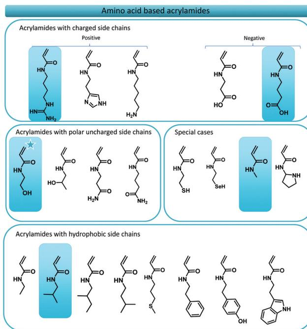
**Fig. 2** Targeted library of amino acid mimicking acrylamides. Each acrylamide displays a functional group that can be found in the 21 natural amino acids. The structure marked with a star is commercially available. The structures indicated with in the blue boxes are the five model monomers investigated in this manuscript.
