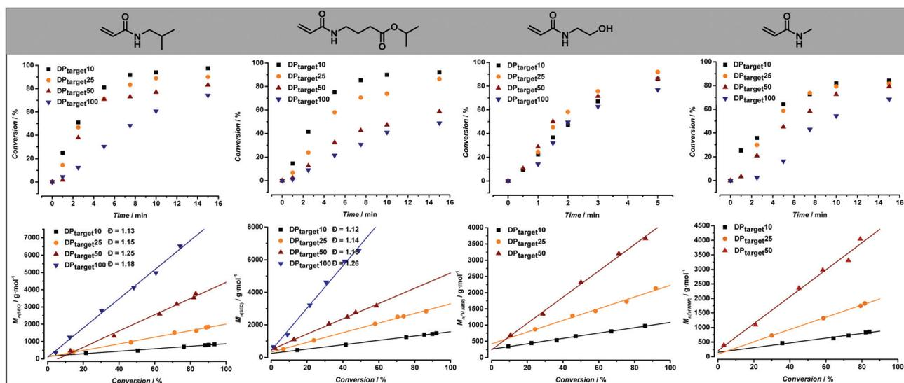
**Fig. 4** Summary of the results obtained from the RAFT polymerization screening reactions of four model monomers. Evolution of monomer conversion over time is given for each monomer in the upper panel of the figure. Number-average molecular weight evolution with conversion under variation of  $[RAFT]/[monomer]$  ratio is given for each monomer in the lower panel of the figure. The best linear fit of the data points is displayed.
