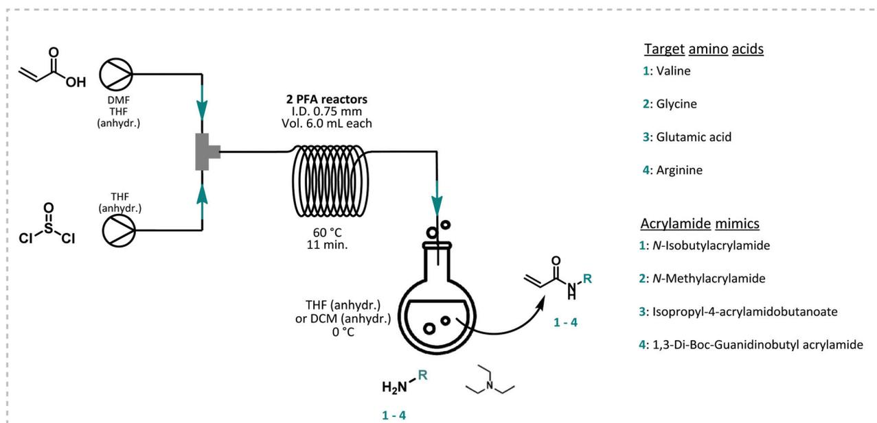
**Fig. 3** Schematic representation of the coupled flow-batch procedure to synthesize four different model acrylamide monomers. In a first step, acryloyl chloride is synthesized in two PFA reactors and without intermediate purification used in the synthesis of a functional acrylamide via a simple nucleophilic addition/elimination reaction with a primary amine in presence of triethylamine (TEA).
