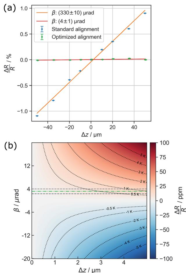
Fig. 1 (a) Minimization of the vergence angle by tuning of electron-optical settings, and (b) the residual impact of the systematic error of the  $z$  displacement on temperature measurements. The dashed dotted line marks the achieved convergence angle shown in (a), whereas the dashed lines show its  $2\sigma$  confidence interval.
