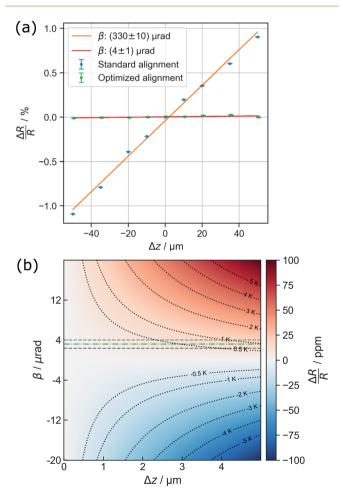
Fig. 1 (a) Minimization of the vergence angle by tuning of electronoptical settings, and (b) the residual impact of the systematic error of the z displacement on temperature measurements. The dashed dotted line marks the achieved convergence angle shown in (a), whereas the dashed lines show its  $2\sigma$  confidence interval
