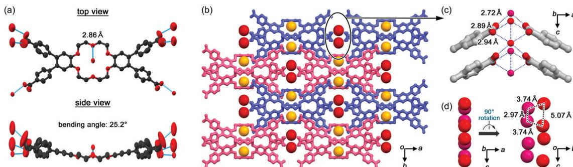
Fig. 3 Crystal structure of **2CT-18C6-III**. (a) Anisotropic ellipsoid plot with 50% probability. (b) Packing diagram, where two types of water molecules are coloured with red and orange. (c) Hydrogen bonds among carboxy groups and water molecules. (d) Alignment of water in the channel with intermolecular distances.
