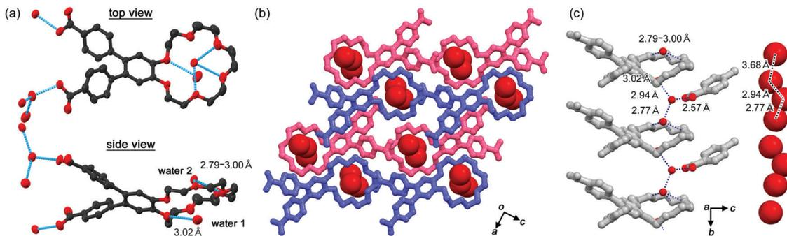
Fig. 4 Crystal structure of **1CT-18C6-I**. (a) Anisotropic ellipsoid plot with 50% probability. (b) Packing diagram, where water molecules are shown by the space-fill model. (c) Hydrogen bonds among the crown ether, carboxy groups, and water molecules. (d) Alignment of water in the channel with intermolecular distances.
