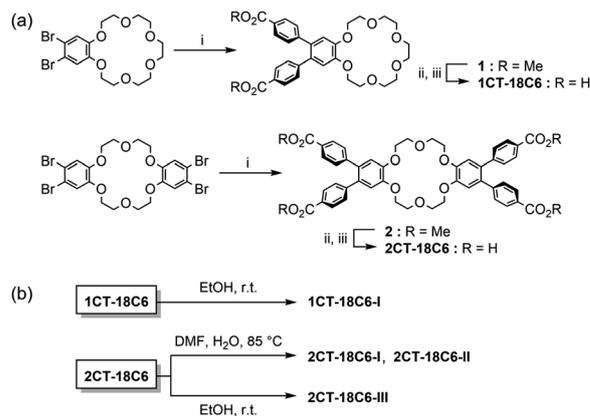
**Scheme 1** (a) Synthesis and (b) crystallization of 1CT-18C6 and 2CT-18C6. Reaction conditions: (i) 4-(methoxycarbonyl)phenylboronic acid,  $\text{Pd}(\text{PPh}_3)_4$ ,  $\text{K}_2\text{CO}_3$ , THF, water, reflux; (ii)  $\text{NaOH}_{\text{aq}}$ , THF, (iii) HCl.
