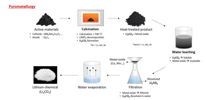
Fig. 7 Overall schematic of lithium recycling from pre-treated waste LIB components by pyrometallurgy process
