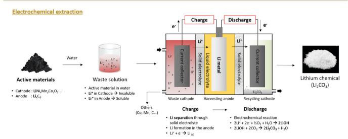
Fig. 9 Overall schematic of lithium recycling from pre-treated waste LIB components by electrochemical extraction process.
