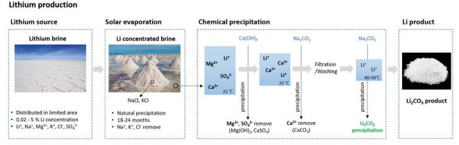
Fig. 2 Process example of Lithium extraction processes from natural lithium brine via chemical precipitation
