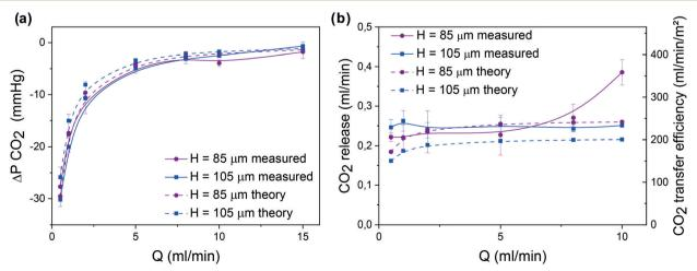
Fig. 5 In vitro performance of single-layer devices under pure oxygen with different heights of blood capillaries ( $H = 85 \mu m$  and  $H = 105 \mu m$ ): (a) variation of the carbon dioxide partial pressure  $\Delta PCO_2$  and (b) the corresponding carbon dioxide release. The theoretical results for the two capillary heights are also represented by dotted lines.
