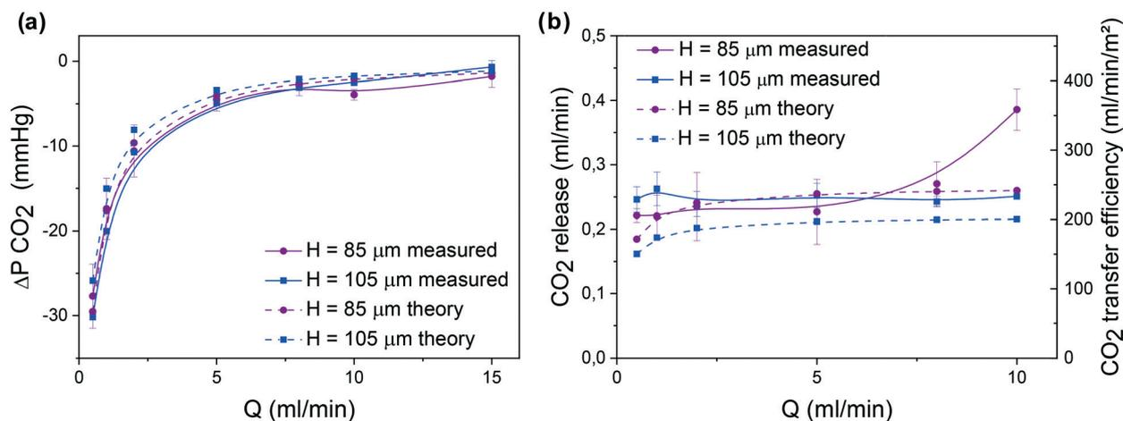
Fig. 5 *In vitro* performance of single-layer devices under pure oxygen with different heights of blood capillaries ( $H = 85 \mu\text{m}$  and  $H = 105 \mu\text{m}$ ): (a) variation of the carbon dioxide partial pressure  $\Delta P \text{ CO}_2$  and (b) the corresponding carbon dioxide release. The theoretical results for the two capillary heights are also represented by dotted lines.
