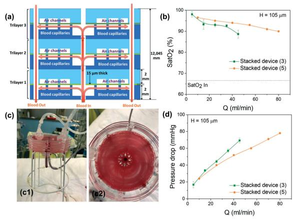
Fig. 6 (a) Cross schematic view of the stacked multilayer device with central blood injection showing the compacity of the whole system and (b) the variation of oxygen saturation level  $Sat(O_2)$  at the output as a function of the blood flow rate for 3- and 5-unit stacked devices. (c) An image of one 5-layer device after measurements (cross view (c1) and top view (c2)). (d) The variation of pressure drop as a function of blood flow rate measured for 3- and 5-unit stacked devices.
