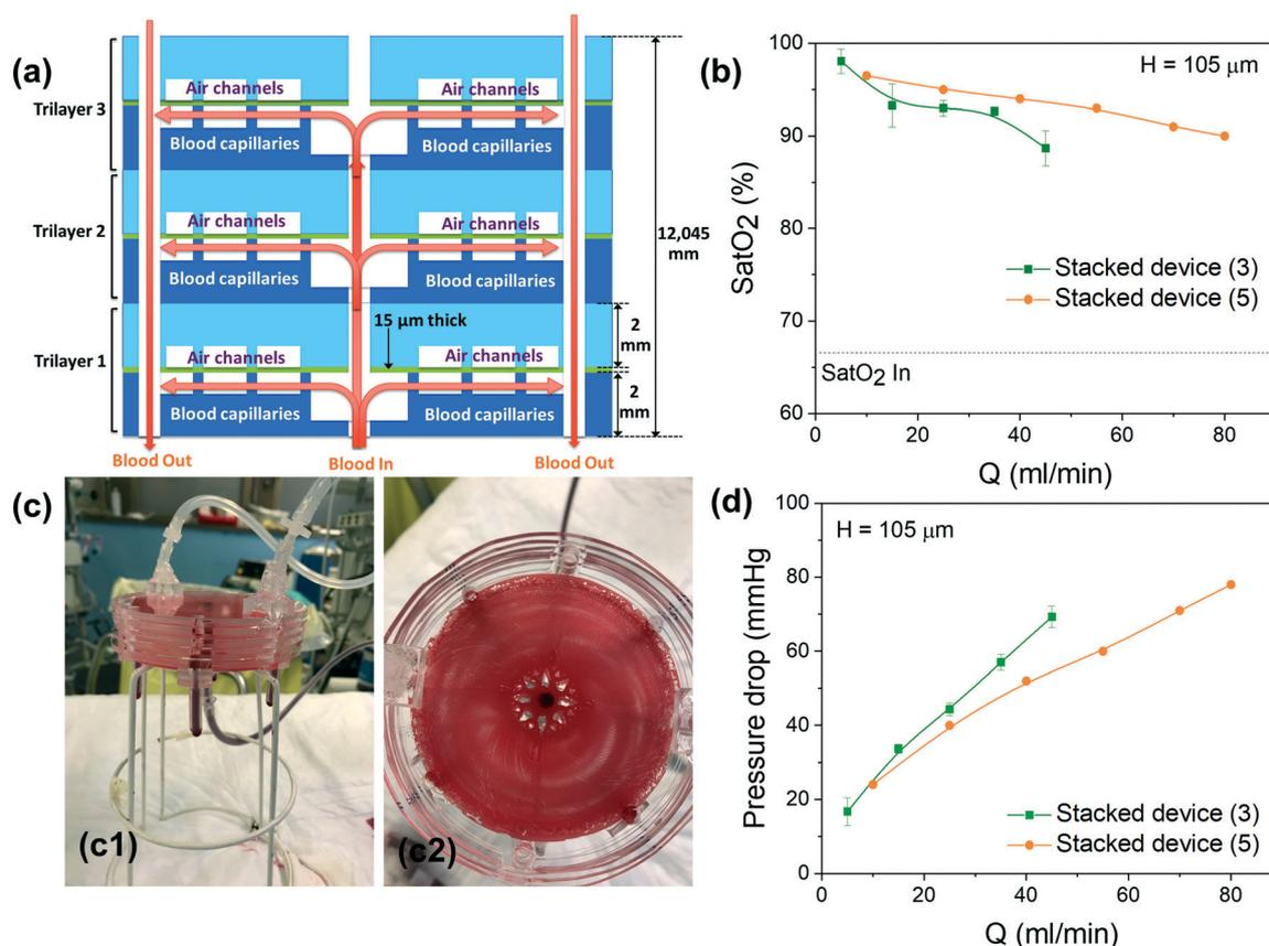
**Fig. 6** (a) Cross schematic view of the stacked multilayer device with central blood injection showing the compacity of the whole system and (b) the variation of oxygen saturation level Sat(O<sub>2</sub>) at the output as a function of the blood flow rate for 3- and 5-unit stacked devices. (c) An image of one 5-layer device after measurements (cross view (c1) and top view (c2)). (d) The variation of pressure drop as a function of blood flow rate measured for 3- and 5-unit stacked devices.
