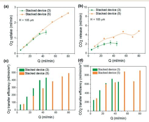
Fig. 7 In vitro performance of stacked devices under pure oxygen (with  $H = 105 \mu m$ ): (a) variation of the oxygen uptake and (b) of the carbon dioxide release as function of the blood flow rate for 3- and 5-unit stacked devices. The corresponding (c) normalized oxygen and (d) carbon dioxide transfer efficiencies as a function of blood flow rate.
