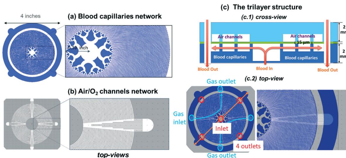
**Fig. 1** Schematic top views of (a) the circular network of blood microcapillaries where blood flows in the white part and (b) the corresponding gas network, (c1) the schematic cross view of one single trilayer structure following the orange arrow in (c2) the top view of the superposed blood and air networks.
