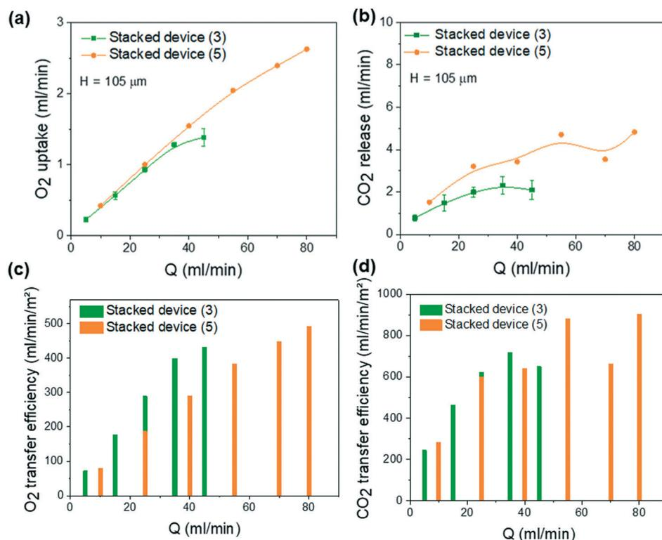
Fig. 7 *In vitro* performance of stacked devices under pure oxygen (with  $H = 105 \mu\text{m}$ ): (a) variation of the oxygen uptake and (b) of the carbon dioxide release as function of the blood flow rate for 3- and 5-unit stacked devices. The corresponding (c) normalized oxygen and (d) carbon dioxide transfer efficiencies as a function of blood flow rate.
