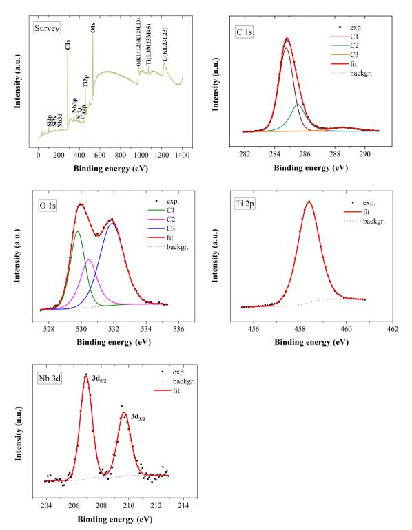
Fig. 5 XPS spectra with the respective survey scan and XPS fits for the C 1s and O 1s core lines for the unused TiO<sub>2</sub>:Nb thin film.
