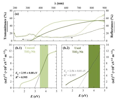
Fig. 7 Representations of the (a) optical transmittance (solid lines) and reflectance (dashed lines) for unused (light green) and used (dark green)  $TiO_2$ :Nb thin film photoanodes over the wavelength ( $\lambda$ ), and (b) Tauc plots for the optical band-gap energy ( $E_g$ ) determination for (b.1) unused and (b.2) used  $TiO_2$ :Nb thin film photoanodes, respectively, with 300 nm thickness.
