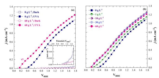
Fig. 9 J-V characteristic curves acquired in a three-electrode "Cappuccino" cell with the fabricated TiO<sub>2</sub>:Nb photoanodes acting as a working electrode at a scan rate of 10 mV s<sup>-1</sup> for (a) 1 M NaOH (pH = 13.2) and 60 g L<sup>-1</sup> lignin (pH = 13.2) aqueous solutions under dark and light conditions, and (b) lignin aqueous solutions at different concentrations (pH = 13.2) under light conditions.
