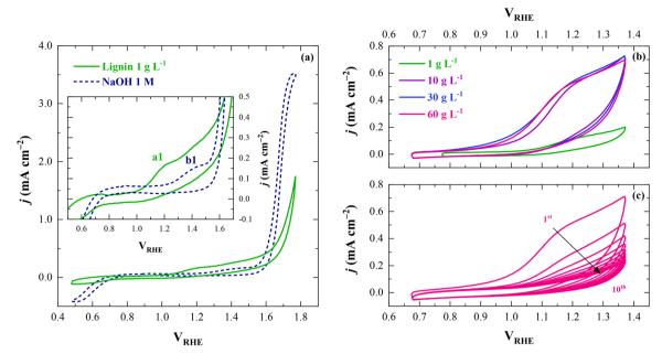
Fig. 8 Cyclic voltammograms acquired in a three-electrode glass cell with a glassy carbon electrode acting as the working electrode at a scan rate of 100 mV s<sup>-1</sup> for (a) 1 M NaOH (pH = 13.2) and 1 g L<sup>-1</sup> lignin (pH = 13.2) aqueous solutions, (b) lignin aqueous solutions at different concentrations (pH = 13.2), and (c) 60 g L<sup>-1</sup> lignin (pH = 13.2) aqueous solution over 10 consecutive cycles.
