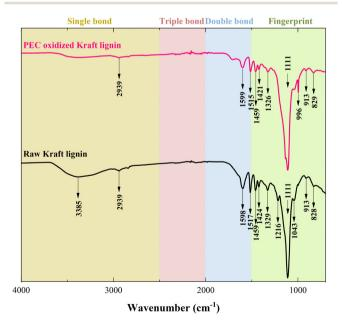
Fig. 2 FT-IR spectra of Kraft lignin before (black line) and after (pink line) photoelectrocatalytic oxidation at  $\sim\!0.8$  V using TiO<sub>2</sub>:Nb photo-anodes for 7 h. Each colored band represents a different region for the occurrence of specific chemical bonds.  $^{48-50}$
