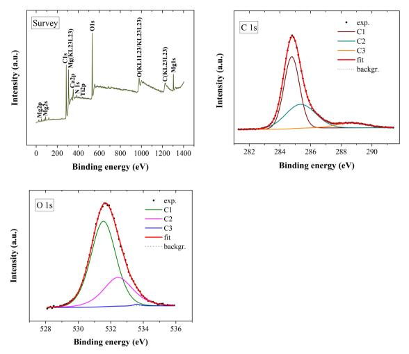
Fig. 6 XPS spectra with the respective survey scan and XPS fits for the C 1s and O 1s core lines for the used TiO₂:Nb thin film.
