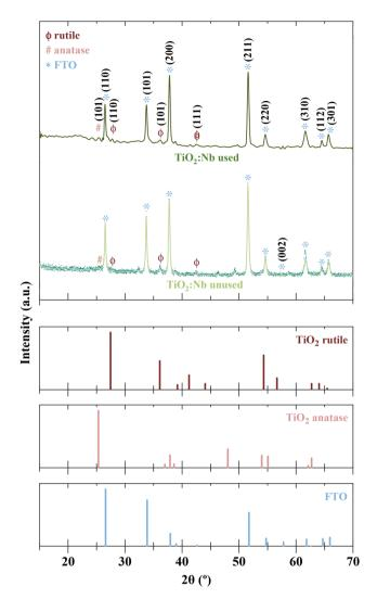
Fig. 4 XRD for the unused and used TiO2:Nb thin films. The XRD patterns (upper graph) were compared with those of TiO2 rutile (ICDD PDF card 00-021-1276), TiO2 anatase (ICDD PDF card 00-064-0863), and SnO<sub>2</sub> (FTO, ICDD PDF cards 00-046-1088 and 01-070-6995). Dotted values indicate experimental data and lines indicate Rietveld refined data.
