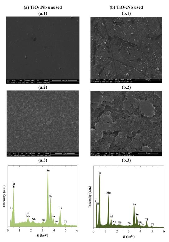
Fig. 3 SEM-EDX analysis of the (a) unused and (b) used TiO<sub>2</sub>:Nb thin films.
