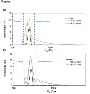
Fig. 3 Molecular weight distributions of the products obtained after 30 min using a 1:1 w/w mixture of p-coumaric and ferulic acids (total mass of 10 mg) in 2 mL of solvent at various conditions in (a) MeOH and (b) EtOH. The result obtained for p-coumaric acid (pCA) is provided as a reference
