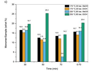
Fig. 5 (a) Yield of monomers (wt%), (b) mass of solvent-soluble products collected (wt%), and (c) monomer/sample ratio (wt/wt%) as a function of time for various operating conditions.
