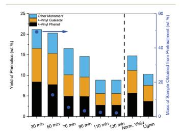
**Fig. 8** Yields of phenolic monomers obtained from fast pyrolysis of lignin and sample depolymerized at 250 °C, 85 bar, EtOH as a function of time. Left *Y*-axis: Yield of phenolic monomers (wt%), Right *Y*-axis: Mass of the solvent-soluble products obtained at corresponding time point from flow-through solvolytic treatment.
