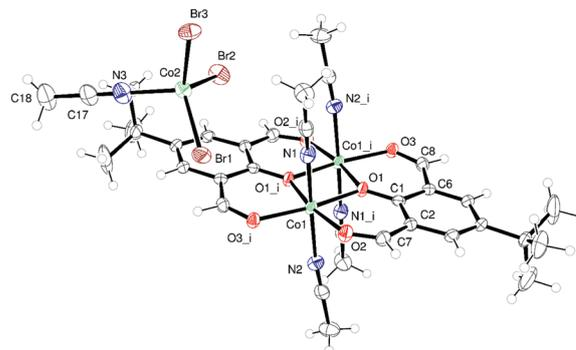
**Fig. 8** Molecular structure of  $[\text{Co}(\text{NCMe})_2\text{L}^5]_2[\text{CoBr}_3(\text{NCMe})_2]$  (**11**) with atoms drawn as 50% probability ellipsoids. Symmetry operation used to generate equivalent atoms:  $i = -x, 1 - y, 1 - z$ . Selected bond lengths (Å) and angles (°): Co(1)–O(1) 2.046(2), Co(1)–O(2) 2.050(2), Co(1)–N(1) 2.108(3), Co(1)–N(2) 2.143(3); O(1)–Co(1)–O(2) 88.56(9), Co(1)–O(2)–Co(1 $_i$ ) 99.59(9), N(1)–Co(1)–N(2) 172.07(11).
