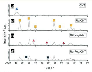
Fig. 2 PXRD-diffractograms of selected catalysts a)-d), measured with  $Cu-K\alpha$  radiation, the blue triangle indicates reflexes for graphitic carbon, the yellow square for RuO2, the red triangle for CuO and the black square for Fe<sub>2</sub>O<sub>3</sub>.
