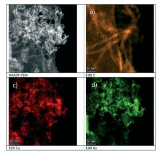
Fig. 1 a) HAADF-TEM image, and EDX elemental mapping images b)-d) of the Ru<sub>2</sub>Cu<sub>1</sub> on CNT catalyst. Additional images can be found in the ESI,† Fig. S2-S5.
