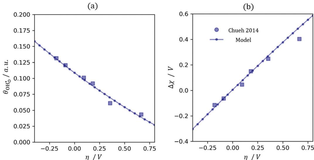
Fig. 5  $\theta_{\text{OH}^*}$  (a) and  $\chi$  (b) on a  $\text{Sm}_{0.2}\text{Ce}_{0.8}\text{O}_{1.9}$ -gas interface as a function of overpotential at 500 °C in 1 : 8 : 4  $\text{H}_2\text{O} : \text{H}_2 : \text{Ar}$ . Squares represent data collected by APXPS measurements (Chueh *et al.*).<sup>29</sup> The dotted and filled lines represent the numerical and analytical solutions to (12), respectively.
