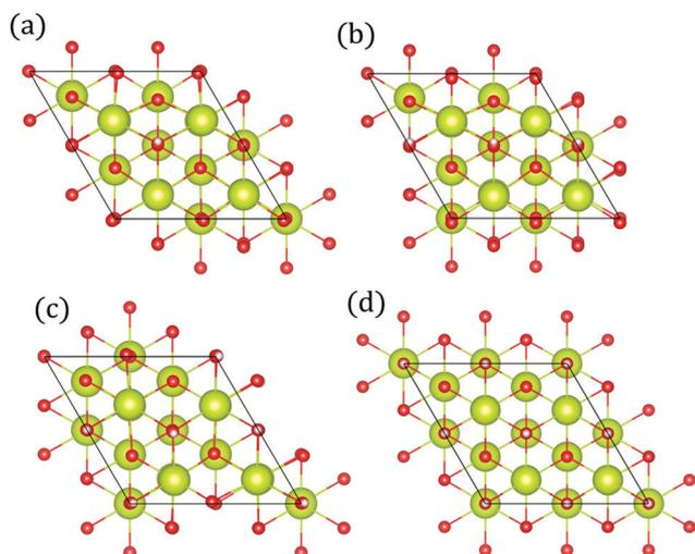
Fig. 2 Structure of lowest energy ceria after surface relaxation. (a)  $\theta_{\text{OH}^*} = 0.25$  with a polaron positioned as the nearest neighbour (NN) with respect to the hydroxyl. (b)  $\theta_{\text{OH}^*} = 0.50$  with polarons positioned NN with respect to the hydroxyls. (c)  $\theta_{\text{OH}^*} = 0.75$  and (d)  $\theta_{\text{OH}^*} = 1.00$ . Ce, O and H atoms are shown as yellow, red and white, respectively.
