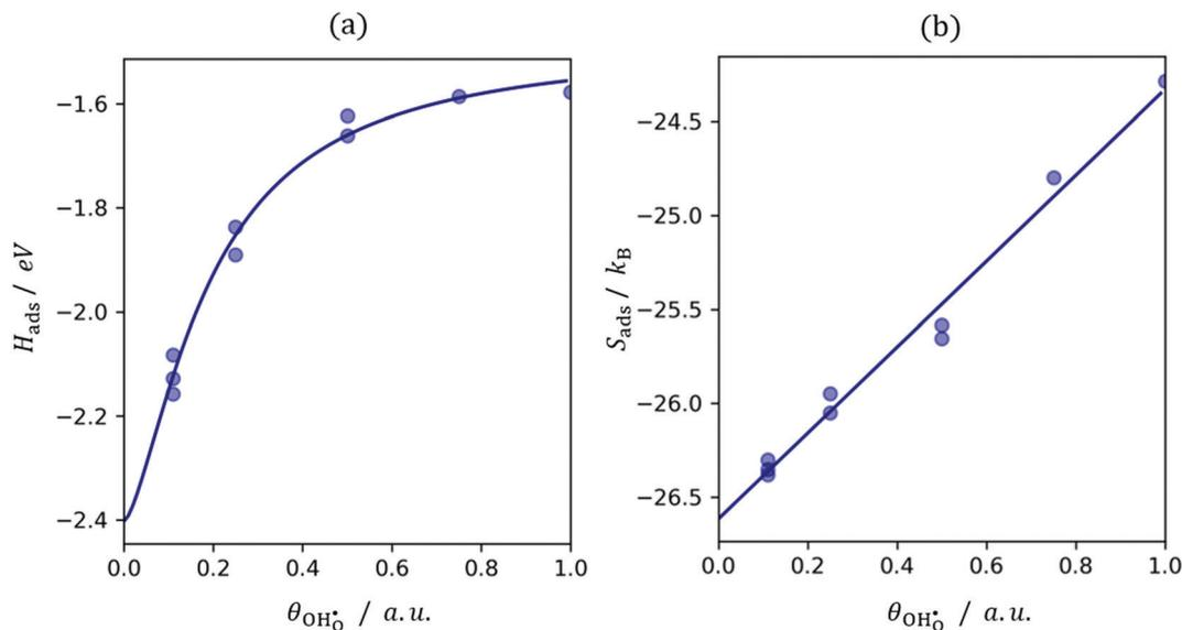
Fig. 4 Hydroxyl coverage dependence on (a) adsorption enthalpy fit to (15) and (b) adsorption entropy with linear fitting.
