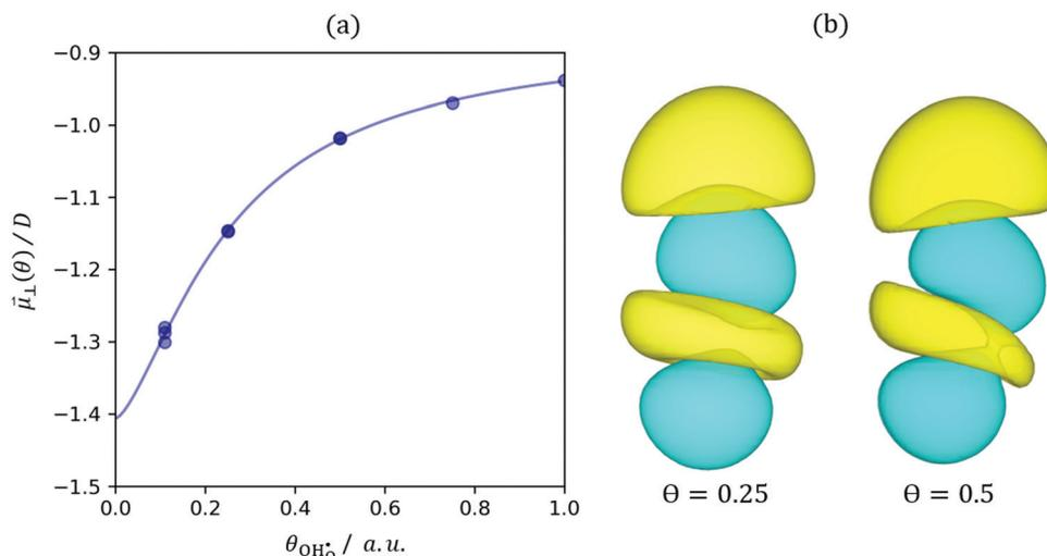
Fig. 3 (a) Calculated hydroxyl dipole moment normal to the ceria[111] termination as a function of coverage. The line fits to eqn (13). (b) Charge density difference isosurface ( $0.005 \text{ Bohr}^{-3}$ ) of the hydroxyl on the ceria surface where negative and positive charge density is represented by blue and yellow isosurfaces, respectively. O site bottom and H site top.
