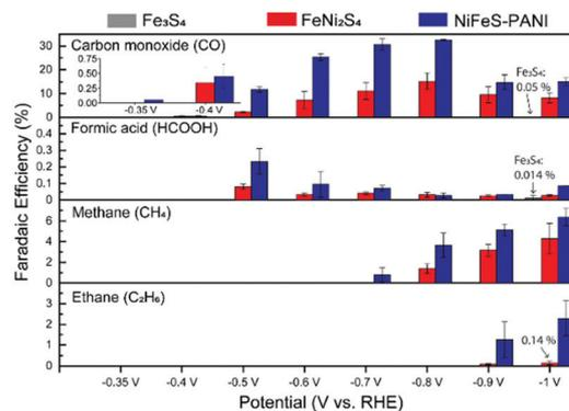
Fig. 1 Performance and analysis of the CO<sub>2</sub> electroreduction products for Fe<sub>3</sub>S<sub>4</sub>, FeNi<sub>2</sub>S<sub>4</sub>, and NiFeS-PANI nanostructures after 4 h of constant potential electrolysis. Calculated FEs are shown for the detected products at each potential. Error bars correspond to the standard error of the mean for at least three independent experiments. FE measurements for Fe<sub>3</sub>S<sub>4</sub> were performed at –0.4, –0.7, and –1.0 V.
