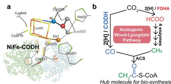
**Scheme 1** (a) The CO<sub>2</sub> molecule interacts with the Ni, Fe, and histidine in the [NiFe<sub>4</sub>S<sub>4</sub>] cluster.<sup>3</sup> (b) The acetogenic W-L pathway converts two molecules of CO<sub>2</sub> into CO and formate, which can be combined to yield the acetyl group of acetyl-CoA.<sup>2b</sup>
