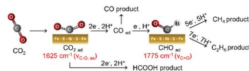
Fig. 4 Proposed pathway for electrochemical  $\text{CO}_2$  reduction to CO, HCOOH,  $\text{CH}_4$ , and  $\text{C}_2\text{H}_6$  on Ni-doped Fe sulfide.
