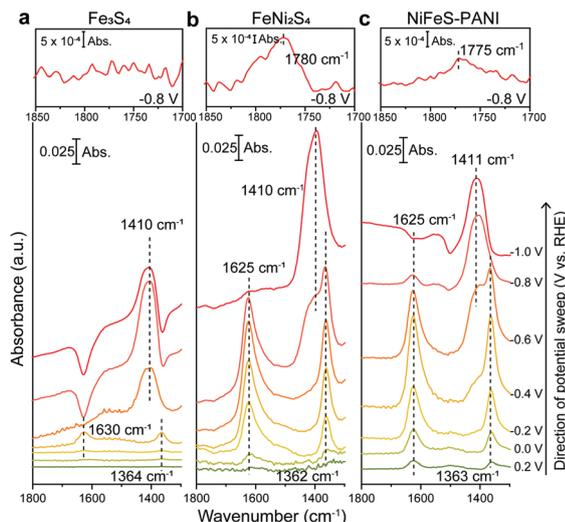
Fig. 2 *In situ* ATR-FTIR spectra of (a)  $\text{Fe}_3\text{S}_4$ , (b)  $\text{FeNi}_2\text{S}_4$ , and (c)  $\text{NiFeS-PANI}$  were recorded during electrochemical  $\text{CO}_2\text{RR}$  in  $\text{CO}_2$ -saturated 0.1 M  $\text{KDCO}_3$ . The insets in the upper panel of (a–c) show magnification of the 1700–1850  $\text{cm}^{-1}$  region at  $-0.8$  V vs. RHE were used as the reference.
