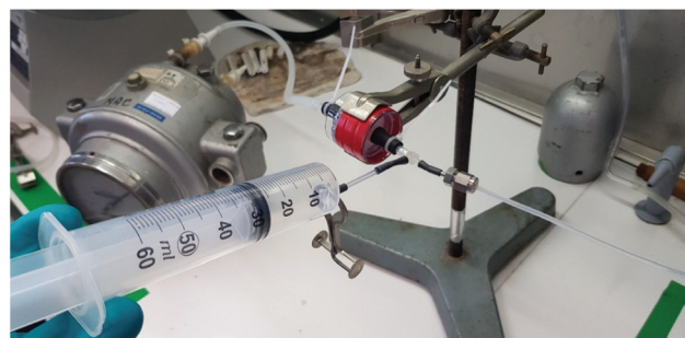
Fig. 8 Gas mixing device and quartz filter trapping system.
