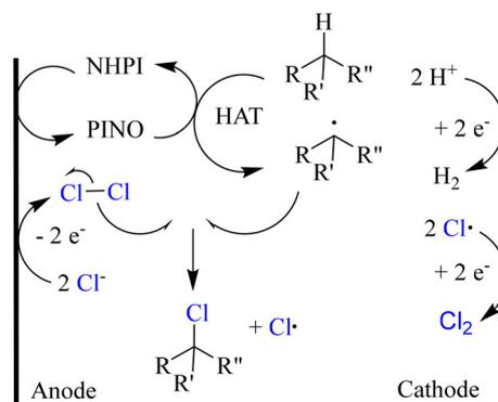
**Scheme 63** Electrochemical chlorination and bromination of benzylic C(sp<sup>3</sup>)-H bonds.
