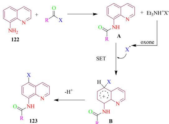
**Scheme 49** One-pot acetylation and C-5 chlorination of 8-aminoquinoline.
