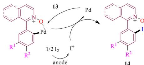
**Scheme 7** Palladium-assisted electrochemical iodination of 1-arylpyridine *N*-oxides.
