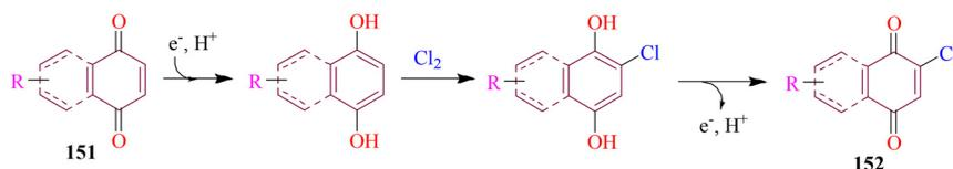
**Scheme 60** Electrochemical chlorination and bromination of different heterocycles.
