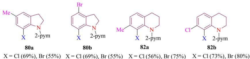
**Scheme 34** Pd-catalyzed chlorination and bromination of indolines and tetrahydroquinolines.
