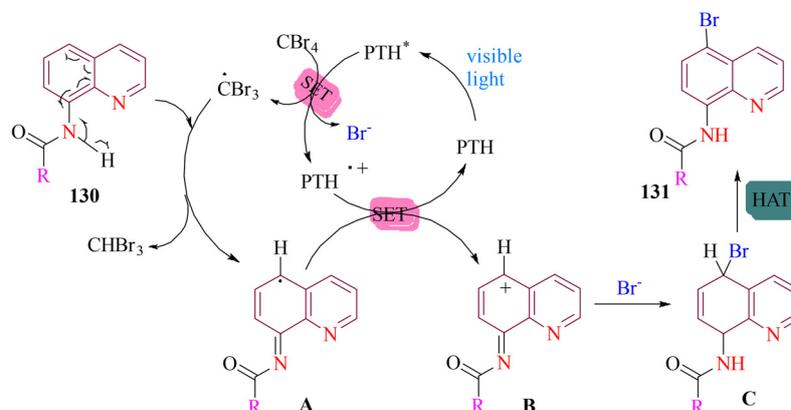
Scheme 52 Organophotocatalyst-mediated C5 bromination of 8-aminoquinoline amides.
