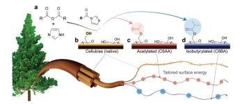
Fig. 1 (a) C6-Regioselective esterification of cellulose in the presence of water. (b) Cellulose with imidazole-catalyzed reaction using (c) acetic or (d) isobutyric anhydrides to yield cellulose nanofibers with tailored surface energy.
