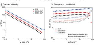
**Fig. 3** Negative contrast SEM images and diameter distribution (lognormal) of native CNF (a and b) and its esterified counterparts, namely C6AA-CNF (c and d) and C6BA-CNF (e and f). Oscillatory rheological profiles of aqueous suspensions (1.5 wt%) of CNF, C6AA-CNF, and C6BA-CNF: (g) flow profiles, and (h) storage and loss moduli.
