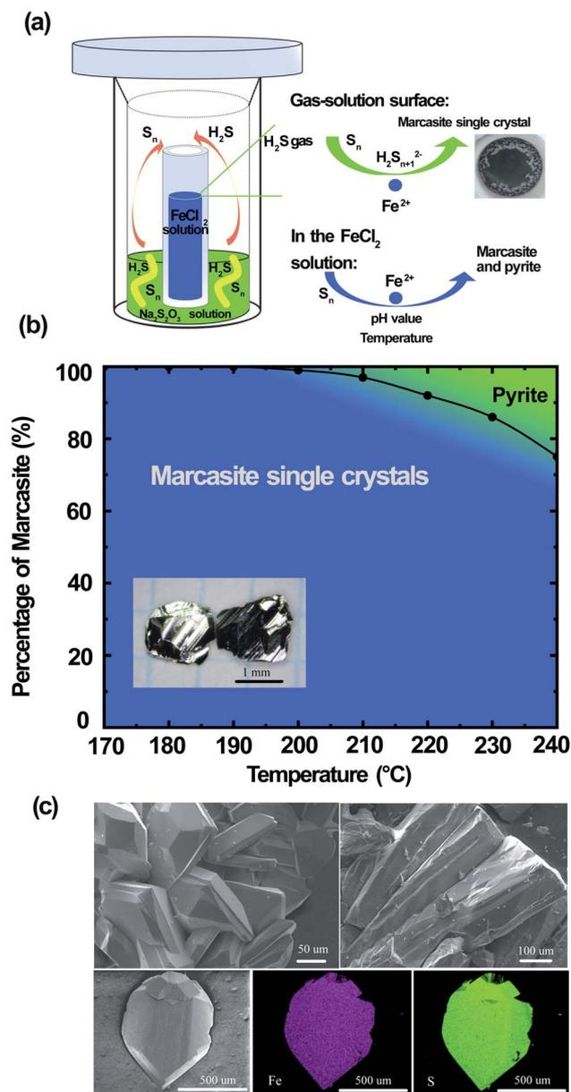
Fig. 3 (a) Space-separated synthesis of FeS<sub>2</sub> marcasite single crystals. (b) Synthesis map of FeS<sub>2</sub> marcasite single crystal and pyrite from the space-separated synthesis. (c) SEM images and EDS mappings of the obtained marcasite crystals.
