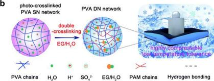
Fig. 7 Two typical synthesis routes of antifreezing organogels: (a) the solvent-exchange method for preparing Ca-alginate/PAAm-Gly, 84 PAMPS/PAAm-EG, 85 gelatin-EG, 102 HPC/PVA-Gly, 55 and TA-CNTs/PVA-Gly organogels. 86 Reproduced with permission from ref. 84, Copyright 2018 Wiley-VCH. (b) In situ polymerization for preparing PVA/PEDOT:PSS-EG,8 PVA/PAAm-EG,74 and PDMA/PEGDMA-heptane organogels.6 Reproduced with permission from ref. 74, Copyright 2020 Royal Society of Chemistry.
