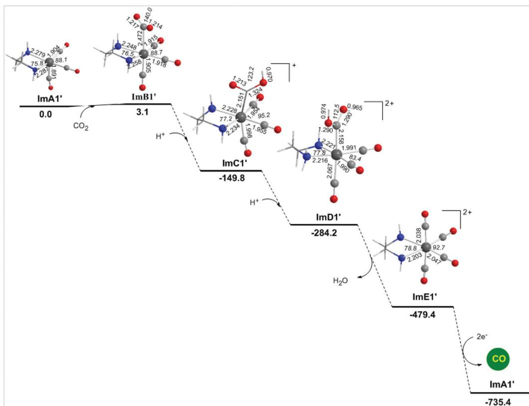
Fig. 5 Geometric and free energy,  $\Delta G$  (in  $\text{kcal mol}^{-1}$ ), reaction profiles for step B1' of the reduction of  $\text{CO}_2$  to  $\text{CO}$  catalyzed by the  $[(\text{en})(\text{CO})_3\text{ReCl}]$  catalyst calculated at the wB97XD/Def2-TZVP level in the DMF solution.
