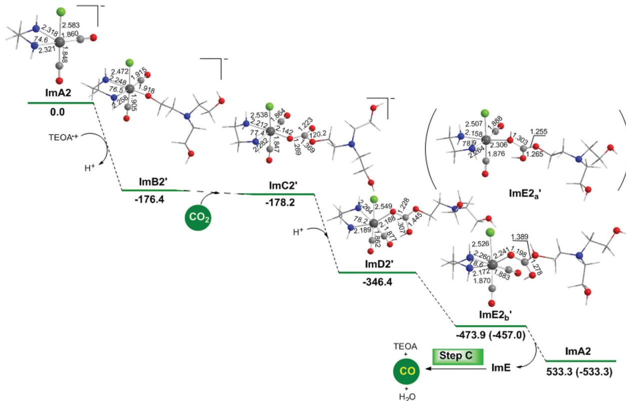
Fig. 8 Geometric and free energy,  $\Delta G$  (in  $\text{kcal mol}^{-1}$ ), reaction profiles for step B2' of the reduction of  $\text{CO}_2$  to CO catalyzed by the active  $[(\text{en})(\text{CO})_3\text{Re}]^-$  catalytic species, **ImA2**, calculated at the wB97XD/Def2-TZVP level in the DMF solution.
