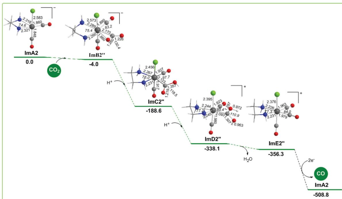
Fig. 9 Geometric and free energy,  $\Delta G$  (in  $\text{kcal mol}^{-1}$ ), reaction profiles for step B2'' of the reduction of  $\text{CO}_2$  to CO catalyzed by the active  $[(\text{en})(\text{CO})_3\text{Re}]^-$  catalytic species, **ImA2**, calculated at the wb97XD/Def2-TZVP level in the DMF solution.
