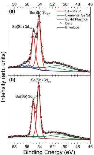
Fig. 4 Se 3d HAXPES data from an Sb<sub>2</sub>Se<sub>3</sub> crystal (a) before and (b) after in situ cleaving.
