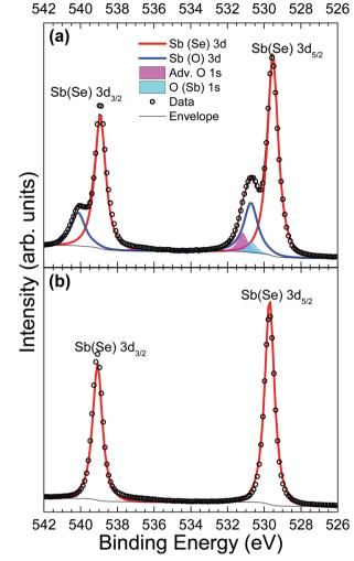
Fig. 3 Sb 3d HAXPES data from an Sb<sub>2</sub>Se<sub>3</sub> crystal (a) before and (b) after in situ cleaving
