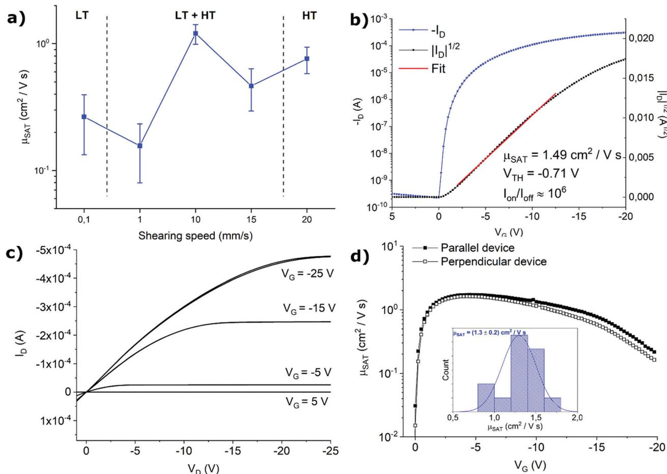
Fig. 4 (a) Mobility vs. shearing speed plot. Representative transfer (b) and output (c) characteristics for a diF-TES-ADT:PS film deposited at  $10 \text{ mm s}^{-1}$ . (d) Mobility profiles for films coated with the channel parallel (filled squares) and perpendicular (empty squares) to the shearing direction (inset: device mobility statistics).
