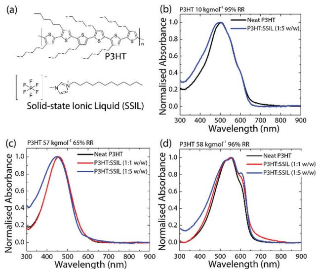
Fig. 1 (a) Chemical structure of the conjugated polymer P3HT and the solid state ionic liquid [C<sub>1</sub>C<sub>12</sub>IM<sup>+</sup>][PF<sub>6</sub><sup>-</sup>] (SSIL). Normalised absorbance spectra of P3HT neat, 1:1 and 1:5 for (b) low  $M_w$  and high RR, (c) high  $M_w$  and low RR and (d) high  $M_w$  and RR P3HT blends.
