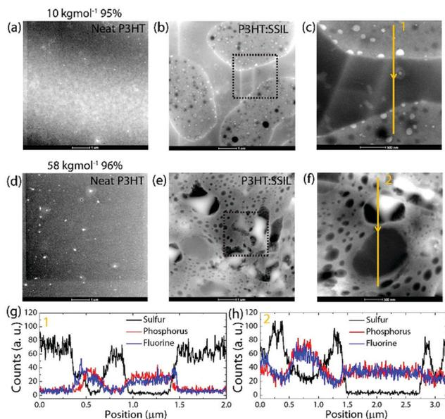
Fig. 3 HAADF-STEM images of P3HT neat and P3HT:SSIL 1 : 1 films: low  $M_w$  P3HT (a) neat and (b) blend, and high  $M_w$  P3HT (d) neat and (e) blend (scale bar: 1  $\mu\text{m}$ ). 1-D elemental profile on the selected region of the low  $M_w$  blend ((1) c and g) and the high  $M_w$  blend ((2) f and h).
