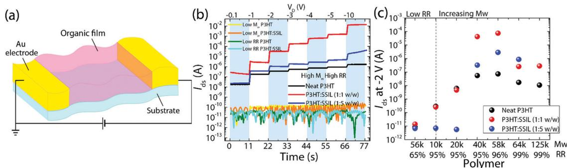
Fig. 2 (a) Diagram of the chemiresistor device structure; (b) driven voltage dependence across the  $L = 5 \mu\text{m}$  and  $W = 2 \text{ mm}$  chemiresistor channel and (c) mean drain current measured for each polymer under an applied bias of  $V_D = -2$  V.
