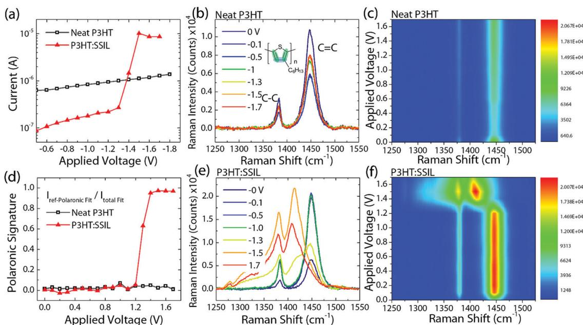
Fig. 5 *In situ* field-dependent Raman spectroscopy (FDRS) of neat P3HT and the P3HT:SSIL 1:1 blend. (a) current measured during FDRS. FDRS for (b) neat P3HT and (e) the P3HT:SSIL blend. 2D Raman intensity plot at different applied voltages for (c) neat P3HT and (f) the P3HT:SSIL blend. (d) Polaronic signature fitted by a linear combination of the reference neutral and polaronic P3HT Raman peaks.
