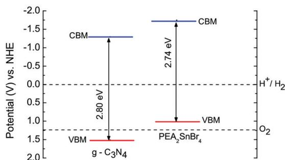
Fig. 4 Calculated band edge positions (solid lines) for two semiconductors relative to NHE potential. The two dashed lines indicate the water redox reaction potentials.
