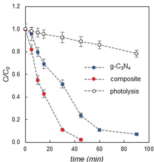
Fig. 3 Variation of MB concentration as a function of irradiation time for g-C<sub>3</sub>N<sub>4</sub> (blue dots) and the PEA<sub>2</sub>SnBr<sub>4</sub>/g-C<sub>3</sub>N<sub>4</sub> 5% composite (red dots), compared to the photolysis effect (empty dots); conditions: 1 g L<sup>-1</sup> catalyst, 250 W m<sup>-2</sup> simulated solar light. RSD < 10% (n = 3).
