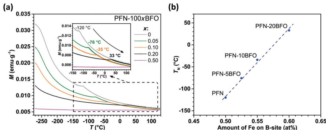
Fig. 2 (a) Temperature dependences of  $M$  for PFN-100xBFO ( $x = 0-0.5$ ) measured at 1 kOe. Inset: The enlarged view of the data between  $-150^{\circ}\text{C}$  and  $120^{\circ}\text{C}$  where  $T_N$  is highlighted. (b) Relationship between  $T_N$  and the amount of Fe on B-site perovskite sublattice for PFN-100xBFO ( $x = 0-0.2$ ).
