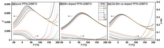
Fig. 4 Temperature and frequency dependences of  $\varepsilon'$  and  $\tan\delta$  of (a) pure, (b) Mn-doped and (c) Gd,Mn co-doped PFN-20BFO
