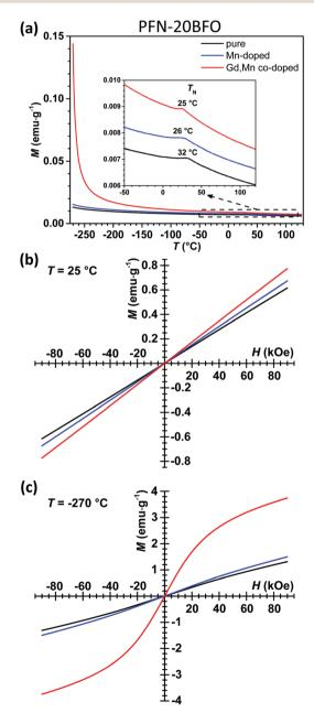
Fig. 6 (a) Temperature dependences of M for PFN–20BFO-based composition measured at 1 kOe. Inset: The enlarged view of the data between  $-50~^{\circ}\text{C}$  and 120  $^{\circ}\text{C}$  where  $T_{\text{N}}$  is highlighted. M-H hysteresis loops of PFN–20BFO-based compositions measured at (b) RT and (c)  $-270~^{\circ}\text{C}$ .
