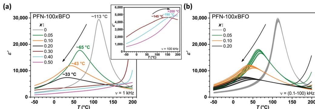
Fig. 1 (a) Temperature dependences of  $\epsilon'$  for PFN-100xBFO measured at 1 kHz ( $x = 0-0.5$ ) and (inset) 100 kHz ( $x \geq 0.3$ ). (b) Temperature and frequency dependence of  $\epsilon'$  for PFN-100xBFO ( $x \leq 0.2$ ) measured in the frequency range of 0.1–100 kHz.
