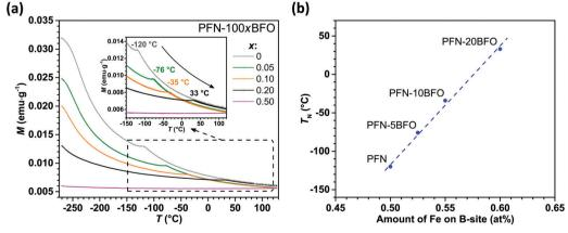
Fig. 2 (a) Temperature dependences of M for PFN-100xBFO (x = 0-0.5) measured at 1 kOe. Inset: The enlarged view of the data between -150 °C and 120 °C where  $T_N$  is highlighted. (b) Relationship between  $T_N$  and the amount of Fe on B-site perovskite sublattice for PFN-100xBFO (x = 0-0.2).
