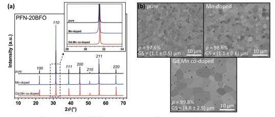
Fig. 3 (a) Room-temperature XRD patterns of PFN-20BFO-based compositions. The indexed peaks of the perovskite phase are labeled according to the cubic notation. The inset shows an enlarged  $2\theta$  region from  $28^{\circ}$  to  $34^{\circ}$ , where no peaks of secondary phases are observed. (b) SEM micrographs of polished PFN-20BFO-based compositions.
