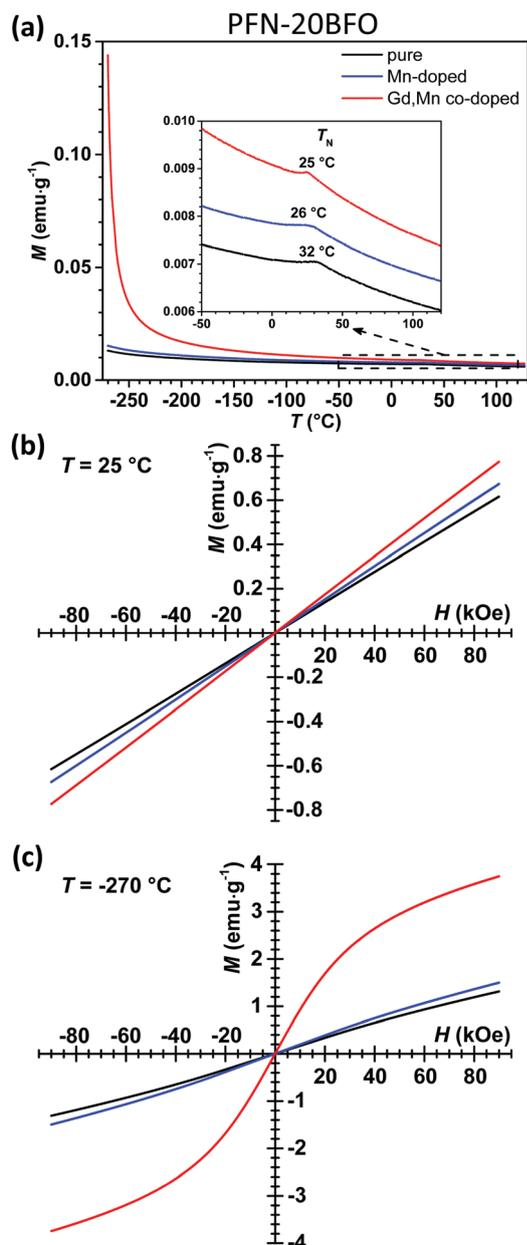
Fig. 6 (a) Temperature dependences of  $M$  for PFN-20BFO-based composition measured at 1 kOe. Inset: The enlarged view of the data between  $-50^\circ\text{C}$  and  $120^\circ\text{C}$  where  $T_N$  is highlighted.  $M$ – $H$  hysteresis loops of PFN-20BFO-based compositions measured at (b) RT and (c)  $-270^\circ\text{C}$ .
