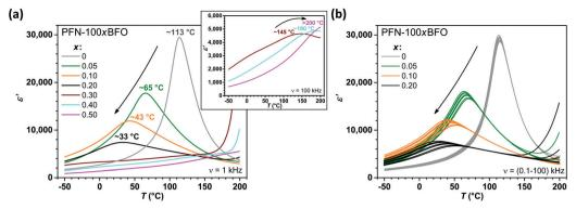
Fig. 1 (a) Temperature dependences of  $\varepsilon'$  for PFN-100xBFO measured at 1 kHz (x = 0-0.5) and (inset) 100 kHz ( $x \ge 0.3$ ). (b) Temperature and frequency dependence of  $\varepsilon'$  for PFN-100xBFO (x  $\leq$  0.2) measured in the frequency range of 0.1-100 kHz.
