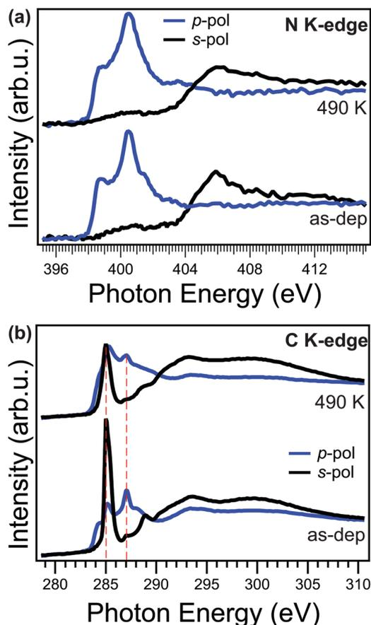
Fig. 4 NEXAFS measurements of the NiTPP/Cu(100) interface. The spectra are acquired at the nitrogen (a) and carbon (b) K-edges for the as-deposited film (bottom panels) and after annealing up to 490 K (top panel).
