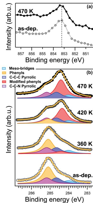
**Fig. 2** XPS spectra of NiTPP/Cu(100) interface at different core level shells. (a) Ni 2p<sub>3/2</sub> spectra of as-deposited (bottom) and annealed up to 470 K (top) film. (b) C 1s spectra (data and fit) of the NiTPP/Cu(100) interface taken after annealing treatment to the indicated temperature. All spectra were collected in normal emission geometry with a photon energy of 1020 (a) and 515 (b) eV, respectively.
