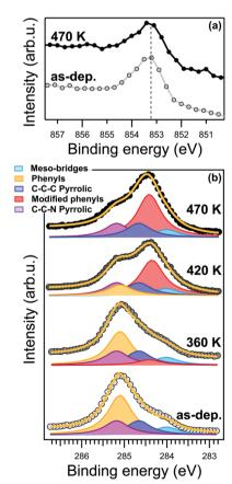
Fig. 2 XPS spectra of NiTPP/Cu(100) interface at different core level shells. (a) Ni  $2p_{3/2}$  spectra of as-deposited (bottom) and annealed up to 470 K (top) film. (b) C 1s spectra (data and fit) of the NiTPP/Cu(100) interface taken after annealing treatment to the indicated temperature. All spectra were collected in normal emission geometry with a photon energy of 1020 (a) and 515 (b) eV, respectively.
