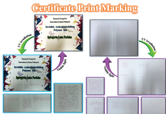
Fig. 10 Application of the stimuli-chromic latex nanoparticles (PMMA-SP) as an anticounterfeiting and rewritable ink for print-marking on security documents.
