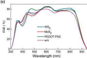
Fig. 3 (a) Molecular structures of PBDB-T-2F, Y6 and PC $_{71}$ BM. (b) J-Vcurves of PBDB-T-2F:Y6:PC71BM based OSCs without a HTL (w/o) and with WS2, MoS2 and PEDOT:PSS as the HTL. Inset: Schematic of the cell architecture. (c) EQE spectra of the cells shown in (b).
