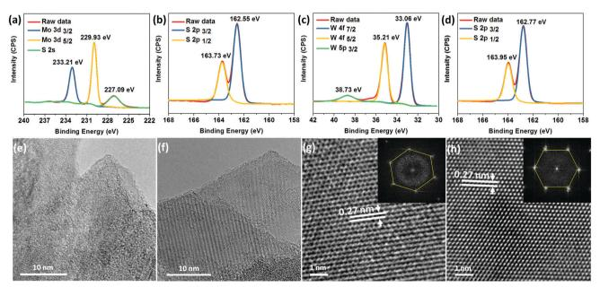
Fig. 2 XPS spectra of the MoS<sub>2</sub> and WS<sub>2</sub> nanosheets deposited on ITO electrodes. (a) Mo3d, (b) S 2p, (c) W 4f, and (d) S 2p regions. TEM images of (e) MoS<sub>2</sub> and (f) WS<sub>2</sub> nanosheets. HRTEM images of (g) MoS<sub>2</sub> and (h) WS<sub>2</sub> with a d-spacing of 0.27 nm corresponding to the (100) plane. Inset: FFT patterns extracted from the HRTEM images, indicating the hexagonal symmetry
