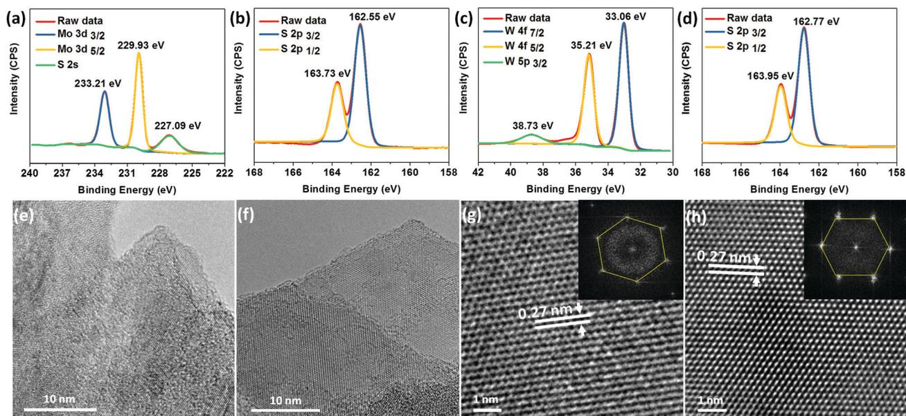
Fig. 2 XPS spectra of the MoS<sub>2</sub> and WS<sub>2</sub> nanosheets deposited on ITO electrodes. (a) Mo 3d, (b) S 2p, (c) W 4f, and (d) S 2p regions. TEM images of (e) MoS<sub>2</sub> and (f) WS<sub>2</sub> nanosheets. HRTEM images of (g) MoS<sub>2</sub> and (h) WS<sub>2</sub> with a *d*-spacing of 0.27 nm corresponding to the (100) plane. Inset: FFT patterns extracted from the HRTEM images, indicating the hexagonal symmetry.
