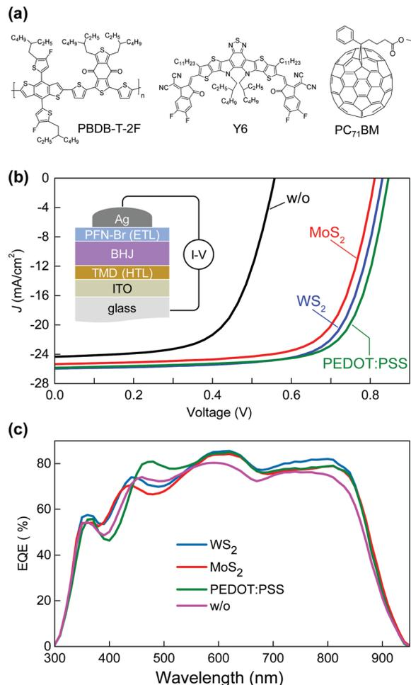
Fig. 3 (a) Molecular structures of PBDB-T-2F, Y6 and PC<sub>71</sub>BM. (b) *J*-*V* curves of PBDB-T-2F:Y6:PC<sub>71</sub>BM based OSCs without a HTL (w/o) and with WS<sub>2</sub>, MoS<sub>2</sub> and PEDOT:PSS as the HTL. Inset: Schematic of the cell architecture. (c) EQE spectra of the cells shown in (b).
