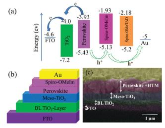
Fig. 3 (a) Energy band diagram of spiro-OMelm; (b) schematic structure of a fully printable mesoscopic perovskite solar cell device using spiro-OMeIm as the HTM; (c) cross sectional SEM image of the active layers of the interfacial junction structure of the device.
