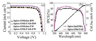
Fig. 7 (a) J-V and IPCE curves for PSCs based on spiro-OMeTAD, spiro-OMeIm and HTMs; (b) the corresponding IPCE spectra for spiro-OMeTAD 1 and spiro-OMelm 2. (FW and BW refer to the forward and backward (reverse) sweeping voltage direction scans respectively)
