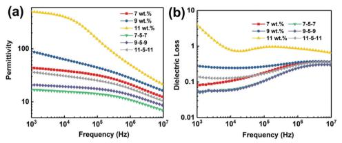
Fig. 5 (a) Dependence of the permittivity and (b) dielectric loss of the single layer and tri-layered composite films
