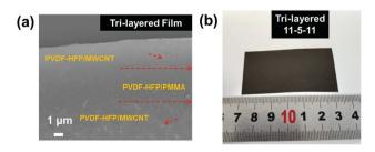
Fig. 3 (a) Cross-section SEM image of the tri-layered composite film with 11 wt% MWCNT and (b) a photograph of the tri-layered composite film
