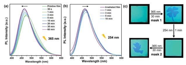
Fig. 6 (a) PL spectra of the P-(Z)-354 film irradiated with 365 nm UV light for different exposure times. (b) PL spectra of the irradiated P-(Z)-354 film further irradiated with 254 nm UV light for different exposure times. (c) Fluorescent pictures of the P-(Z)-345 film irradiated with 365 nm UV light and then with 254 nm light.
