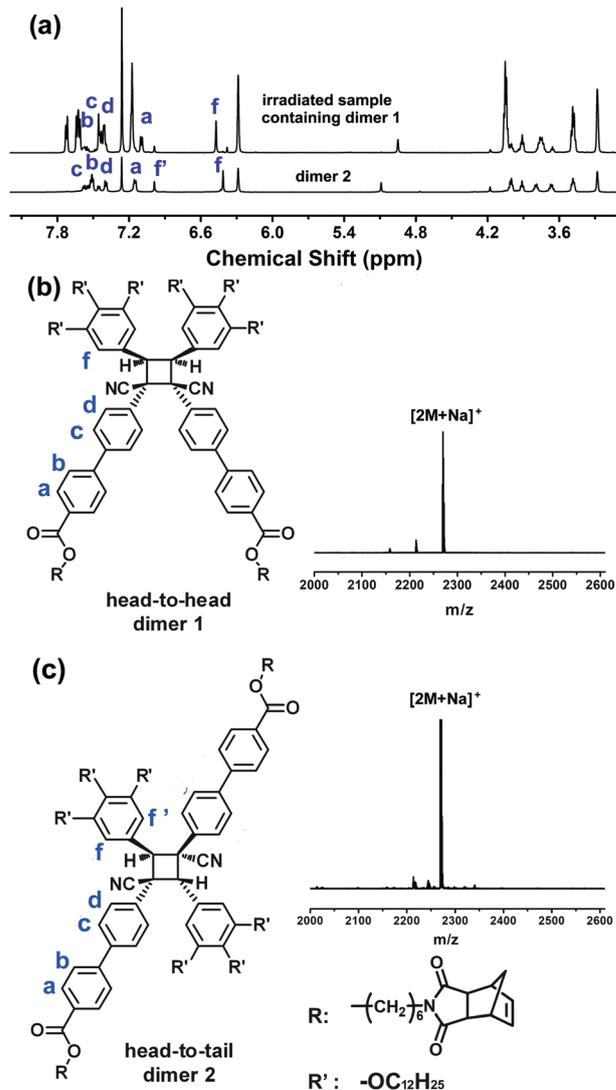
Fig. 8 (a) <sup>1</sup>H NMR spectra of the irradiated sample containing dimer 1 and purified dimer 2.; Chemical structures and corresponding MS spectra of dimer 1 (b) and dimer 2 (c).
