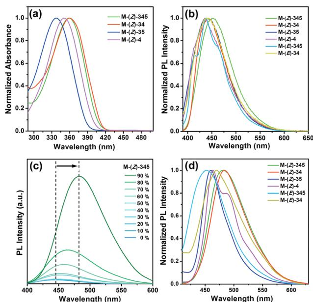
Fig. 4 (a) UV-vis absorption spectra of monomers in CHCl<sub>3</sub> ( $1 \times 10^{-5}$  mol L<sup>-1</sup>). (b) PL spectra of monomers in CHCl<sub>3</sub> ( $1 \times 10^{-5}$  mol L<sup>-1</sup>). (c) PL spectra changes of M-(Z)-345 depending on the water fractions in THF. (d) Fluorescence spectra of monomers in the solid state.
