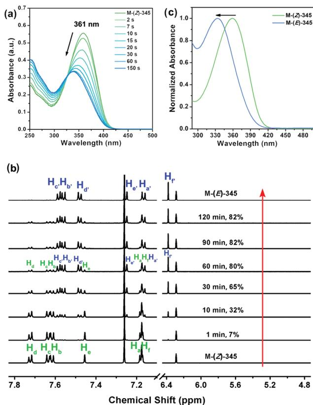
Fig. 1 (a) UV-vis absorption spectra of *M*-(*Z*)-345 in  $\text{CHCl}_3$  ( $1 \times 10^{-5} \text{ mol L}^{-1}$ ) before and after irradiation upon 365 nm UV light with increasing illumination times; (b)  $^1\text{H}$  NMR spectra of *M*-(*Z*)-345 before and after 365 nm UV irradiation with different illumination times and pure *M*-(*E*)-345; (c) UV-vis absorption spectra of pure *M*-(*Z*)-345 and *M*-(*E*)-345 in  $\text{CHCl}_3$  solution.
