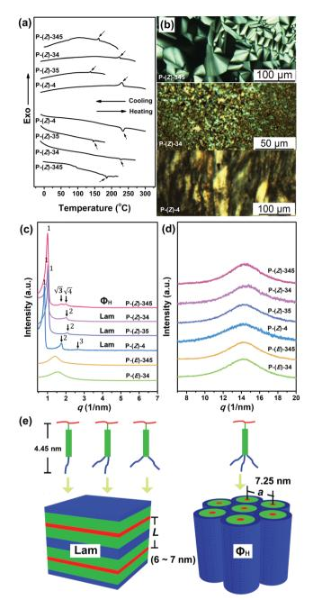
Fig. 3 (a) DSC curves of polymers at a heating and cooling rate of 10 °C min $^{-1}$ . (b) POM pictures of P-(Z)-345 at 150 °C, P-(Z)-34 at 201 °C and P-(Z)-4 at 210 °C. SAXS (c) and WAXS (d) profiles of thermally annealed polymers recorded at room temperature. (e) schematic illustration of the phase structure model of smectic and  $\Phi_H$  phases.
