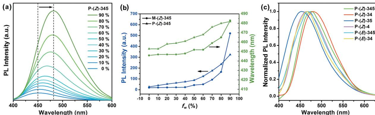
Fig. 5 (a) PL spectral changes of P-(Z)-345 depending on the water fractions in THF. (b) PL intensity and wavelength of M-(Z)-345 and P-(Z)-345 as a function of water content ( $f_w$ ) in THF/water mixtures. (c) PL spectra of polymer films.
