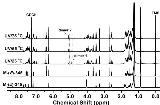
Fig. 7 <sup>1</sup>H NMR spectra of M-(Z)-345, M-(E)-345 and the as-casted film of M-(Z)-345 irradiated with 365 nm UV light at 25, 55 and 75 °C for 30 min.
