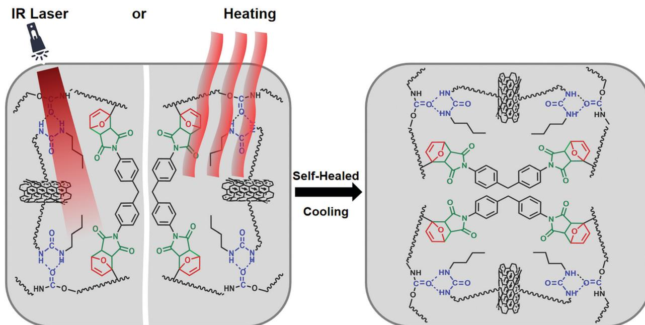
Fig. 6 Illustration of self-healing process of RCFA.
