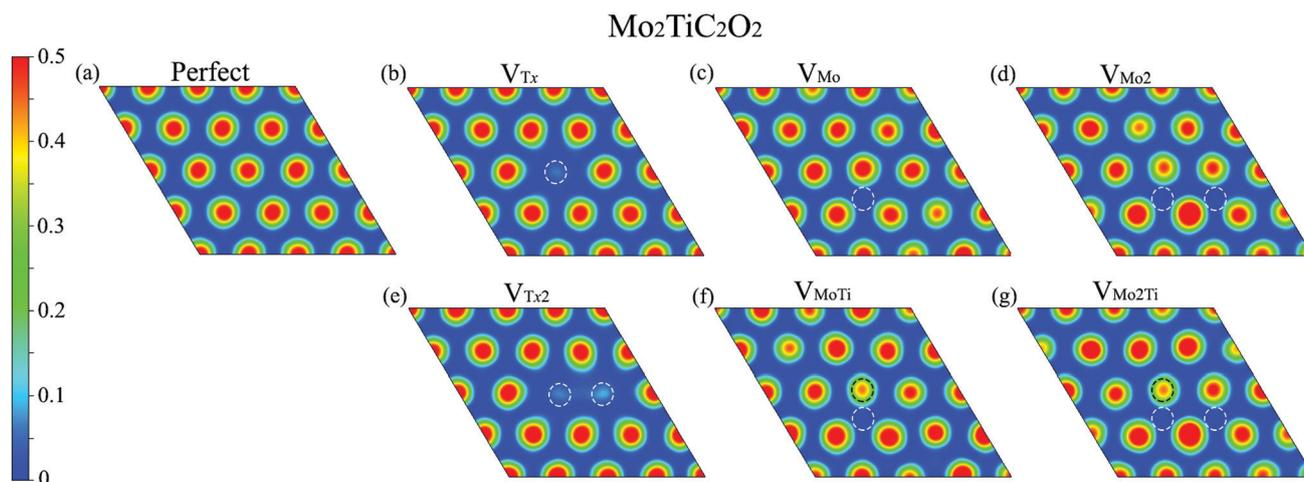
Fig. 6 Electron localization function (ELF) on the plane perpendicular to the  $c$ -axis at a close distance on top of surface terminations of the defected  $\text{Mo}_2\text{TiC}_2\text{O}_2$  MXenes. Dashed circle lines highlight the place of the removed atoms.
