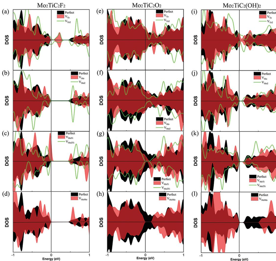
Fig. 4 Effect of different types of defects on the DOS of MXenes with different terminations. (a–d)  $\text{Mo}_2\text{TiC}_2\text{F}_2$ , (e–h)  $\text{Mo}_2\text{TiC}_2\text{O}_2$ , and (i–l)  $\text{Mo}_2\text{TiC}_2(\text{OH})_2$ . The type of defect is shown in the different panels.
