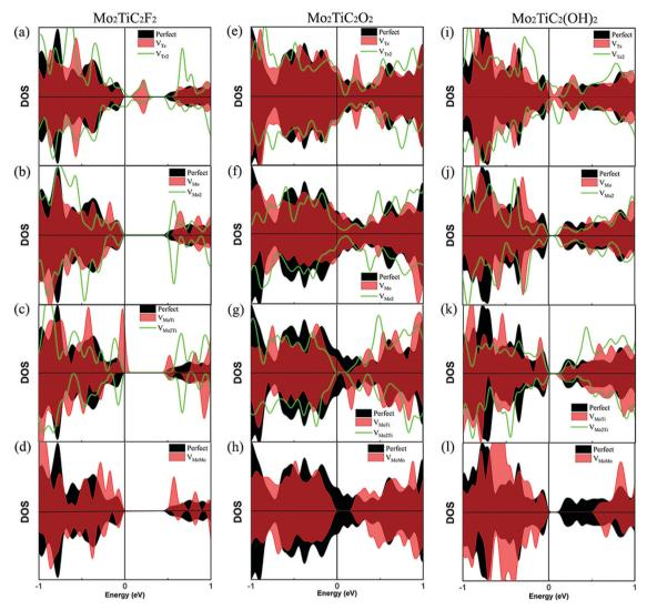
Fig. 4 Effect of different types of defects on the DOS of MXenes with different terminations. (a–d) Mo<sub>2</sub>TiC<sub>2</sub>F<sub>2</sub>, (e–h) Mo<sub>2</sub>TiC<sub>2</sub>O<sub>2</sub>, and (i–l) Mo<sub>2</sub>TiC<sub>2</sub>(OH)<sub>2</sub>. The type of defect is shown in the different panels.
