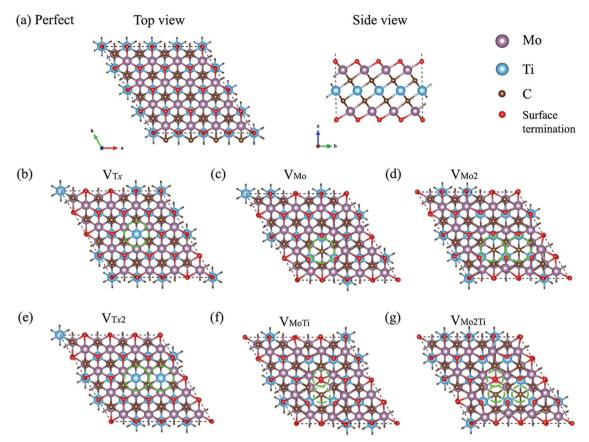
Fig. 1 Fully relaxed structural models of different types of defects considered in monolayer ordered  $Mo_2TiC_2T_{x\cdot}$  (a) Top and side view of the perfect MXene. Top views of (b)  $V_{T_u}$ , (c)  $V_{Mo}$ , (d)  $V_{Mo_2}$ , (e)  $V_{T_u2}$ , (f)  $V_{MoTi}$ , and (g)  $V_{Mo_2Ti}$ .
