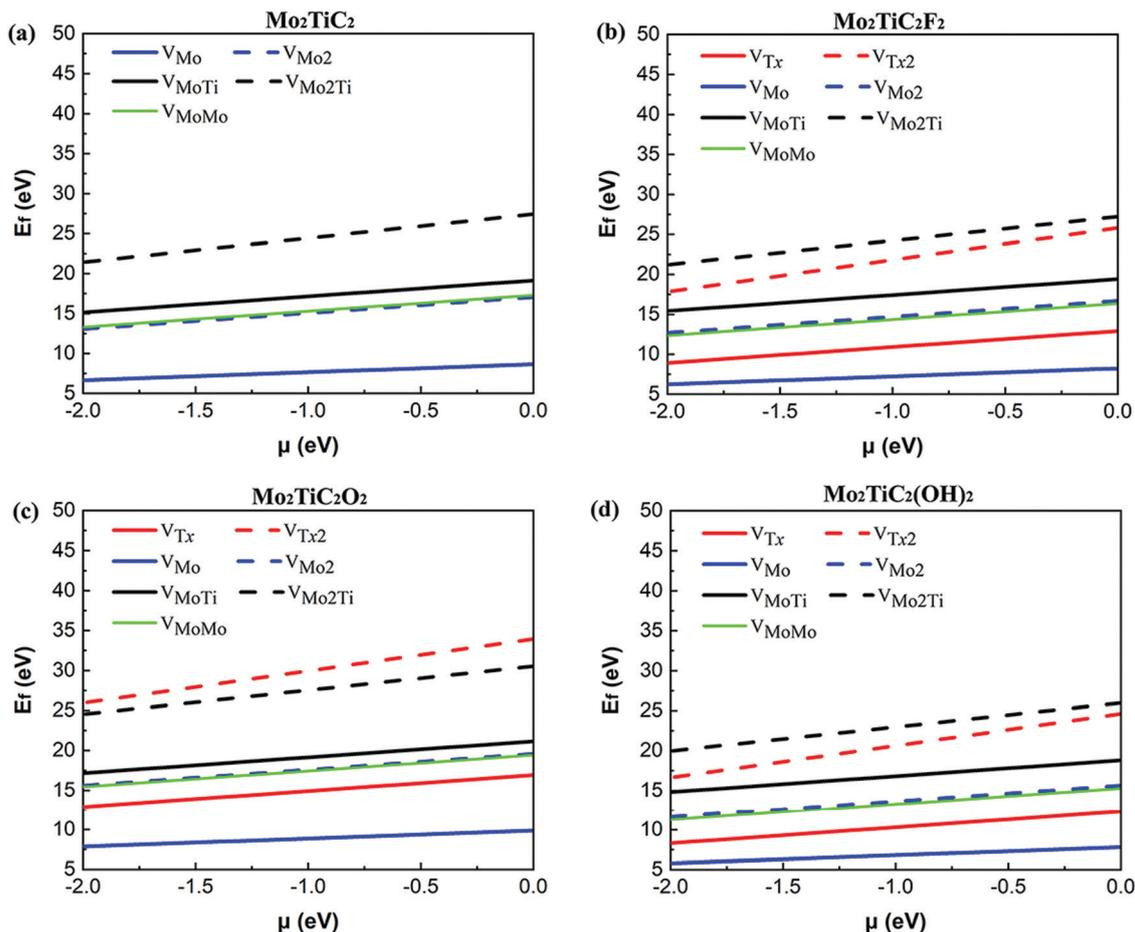
Fig. 2 Formation energies of all types of defects as a function of the chemical potential of the removed atom(s) in the range of  $-2 \text{ eV} < \mu < 0 \text{ eV}$  in (a)  $\text{Mo}_2\text{TiC}_2$ , (b)  $\text{Mo}_2\text{TiC}_2\text{F}_2$ , (c)  $\text{Mo}_2\text{TiC}_2\text{O}_2$ , (d) and  $\text{Mo}_2\text{TiC}_2(\text{OH})_2$ .
