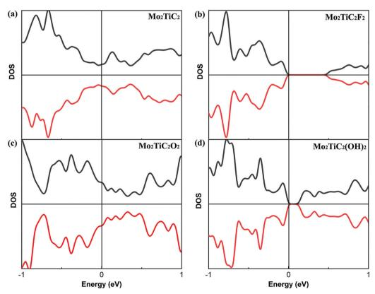
Fig. 3 Calculated total density of states (DOS) of perfect MXenes. (a) Pristine MXene, (b)  $Mo_2TiC_2F_2$ , (c)  $MoTiC_2O_2$ , and (d)  $Mo_2TiC_2(OH)_2$ . Black and red lines show spin-up and -down states, respectively.
