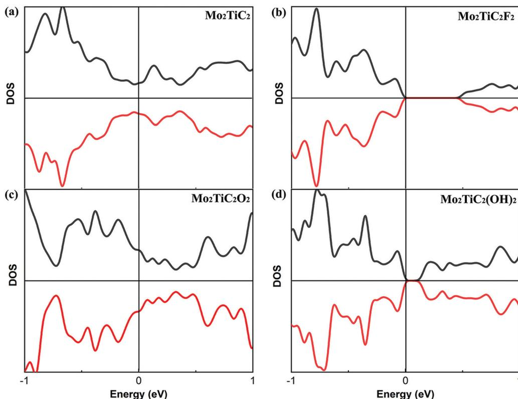
Fig. 3 Calculated total density of states (DOS) of perfect MXenes. (a) Pristine MXene, (b)  $\text{Mo}_2\text{TiC}_2\text{F}_2$ , (c)  $\text{Mo}_2\text{TiC}_2\text{O}_2$ , and (d)  $\text{Mo}_2\text{TiC}_2(\text{OH})_2$ . Black and red lines show spin-up and -down states, respectively.
