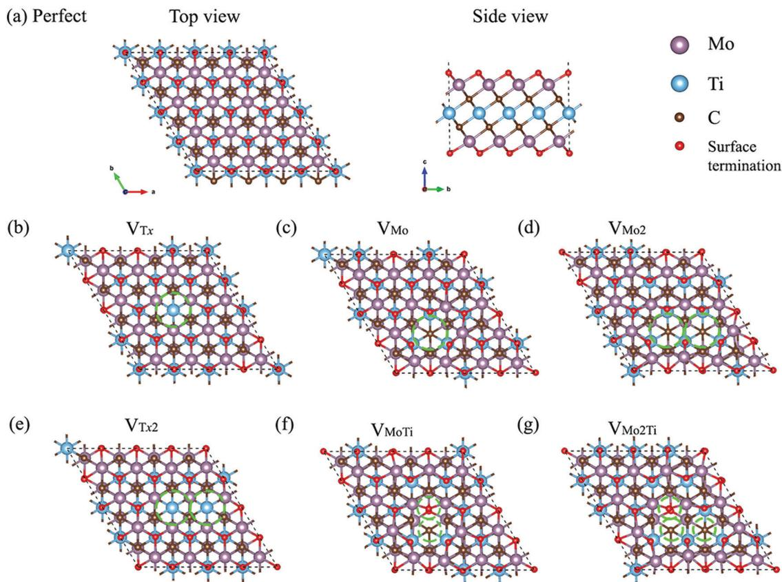
Fig. 1 Fully relaxed structural models of different types of defects considered in monolayer ordered  $\text{Mo}_2\text{TiC}_2\text{T}_x$ . (a) Top and side view of the perfect MXene. Top views of (b)  $\text{V}_{\text{T}_x}$ , (c)  $\text{V}_{\text{Mo}}$ , (d)  $\text{V}_{\text{Mo}_2}$ , (e)  $\text{V}_{\text{T}_x2}$ , (f)  $\text{V}_{\text{MoTi}}$ , and (g)  $\text{V}_{\text{Mo}_2\text{Ti}}$ .
