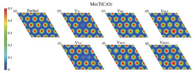
Fig. 6 Electron localization function (ELF) on the plane perpendicular to the c-axis at a close distance on top of surface terminations of the defected Mo<sub>2</sub>TiC<sub>2</sub>O<sub>2</sub> MXenes. Dashed circle lines highlight the place of the removed atoms.
