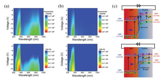
Fig. 3 (a) Photoresponsivity (top) and EQE (bottom) pseudo-color maps of this heterojunction photodiode measured under reverse bias voltages. (b) Photoresponsivity (top) and EQE (bottom) pseudo-color maps of this heterojunction photodiode measured under forward bias voltages. (c) Schematic energy band diagram showing the band alignment and carrier dynamics of this device operating under reverse bias (top) and forward bias (bottom) conditions
