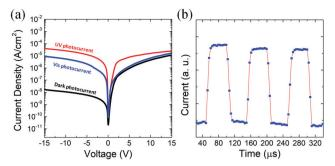
Fig. 2 (a) I-V characteristics of the photodetector measured in the dark, under 760 nm visible illumination, and 375 nm UV illumination. (b) Transient response of the heterojunction photodiode with a rising time of 4.3 µs and a falling time of 5.2 µs measured under ambient conditions.
