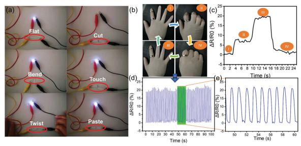
Fig. 5 Photographs demonstrating the electrical conductivity of the ion gel with various deformations (a). The ion gel as electronic skin to monitor the grasping motion (b) and its corresponding current change (c). Relative resistance changes of the ion gel as a wearable sensor in monitoring finger bending motion (d and e).
