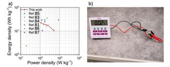
Fig. 7 Ragone plots of the EDLC with the DES-based ion gel electrolyte and some of the reported values of ionic liquid-based ion gel electrolytes (a), and the EDLC fabricated with the DP3 ion gel as the power source of a clock (b).
