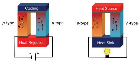
Fig. 4 A representation of the TE effect in (left) a Peltier cooler and (right) a TE generator. Charge carriers move from one end of the thermocouple, carrying entropy and heat towards the other end. Both n- and p-type materials are necessary for a complete device.
