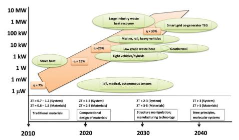
Fig. 11 A Roadmap for the exploitation of thermoelectric technology, where ZT is the thermoelectric figure of merit and  $\eta$  the efficiency.
