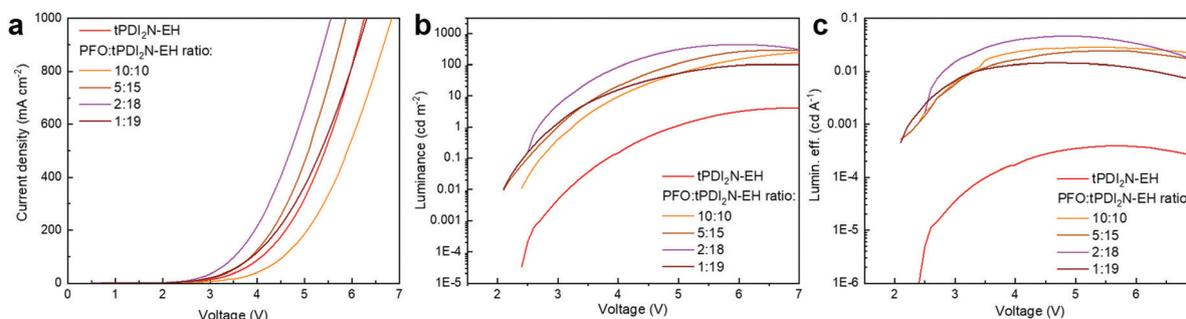
Fig. 3 (a) Current density–voltage ( $J$ – $V$ ) characteristics, (b) luminance *versus* applied voltage ( $L$ – $V$ ,  $\text{cd m}^{-2}$ ) and (c) luminous efficiency (lumin. eff.) *versus* current density ( $LE$ – $J$ ,  $\text{cd A}^{-1}$ ) of PFO:tPDI<sub>2</sub>N-EH OLEDs at selected ratios.
