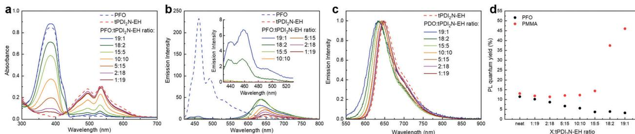
**Fig. 2** (a) Optical absorption and (b and c) photoluminescence spectra of PFO:tPDI<sub>2</sub>N-EH-blend and neat films spin-cast from toluene at 15 mg mL<sup>-1</sup> under (b)  $\lambda_{\text{ex}} = 400$  nm and (c)  $\lambda_{\text{ex}} = 530$  nm. (d) PL quantum yield (QY) values of X:tPDI<sub>2</sub>N-EH (X = PFO or PMMA) blend films with different ratio. Excitation wavelengths for PLQY measurements was 530 nm.
