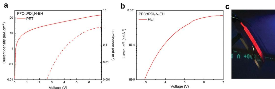
Fig. 5 (a) Current–voltage–luminance characteristics and (b) luminous efficiency (lumin. eff.) versus current density ( $LE-J$ ,  $cd A^{-1}$ ) of PFO:tPDI<sub>2</sub>N-EH roll-to-roll coated on PET. (c) Photo of electroluminescent of PFO:tPDI<sub>2</sub>N-EH OLEDs on PET.
