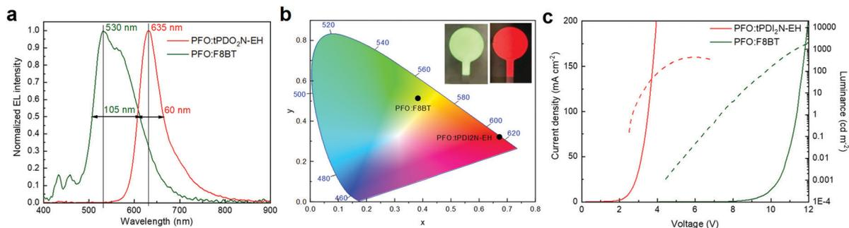
Fig. 4 (a) Normalized electroluminescence (EL) and (b) color coordinates spectra, (c) current–voltage–luminance characteristics of PFO:F8BT (ratio 19:1) and PFO:tPDI<sub>2</sub>N-EH (ratio 2:18) blends.
