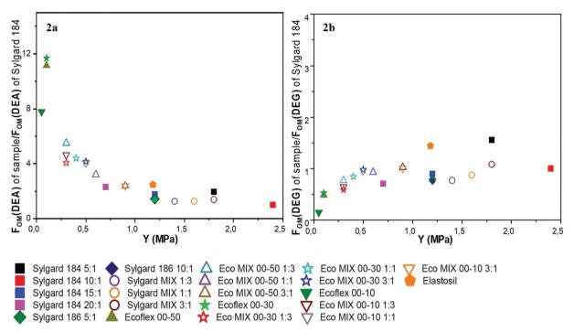
Fig. 2 Figures of merit (a) for actuator ( $F_{om}(DEA)$ ) and (b) for generator ( $F_{om}(DEG)$ ), both normalized with Sylgard 184. For the calculations, e' is measured at 1 Hz and  $\phi$  calculated from hysteresis curves
