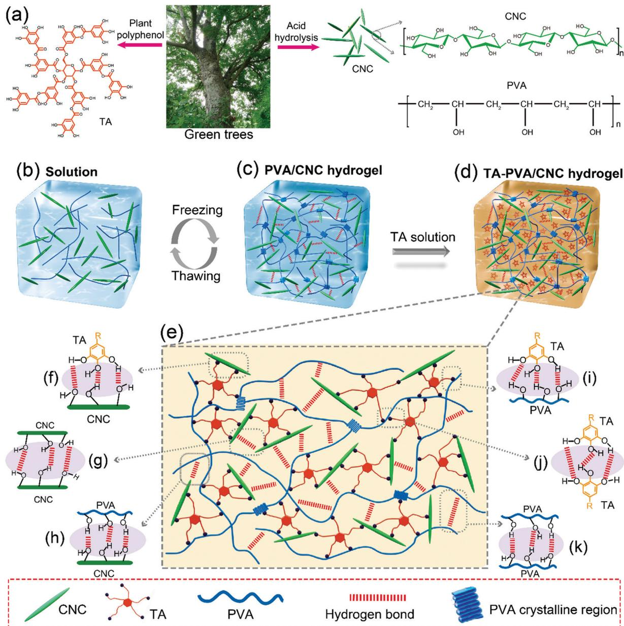
**Scheme 1** (a) Chemical structure of TA, CNC and PVA. (b–e) Illustration of the fabrication of TA–PVA/CNC hydrogels and their possible formation mechanism. (f–k) The hydrogen bonds between TA and CNC, CNC and CNC, PVA and CNC, TA and PVA, TA and TA, as well as PVA and PVA, respectively.
