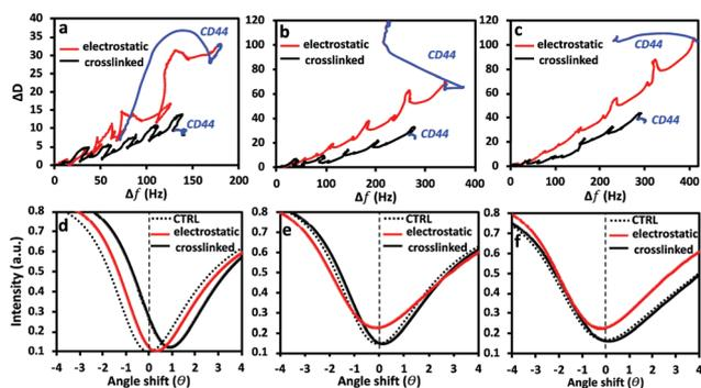
Fig. 5 (a–c) QCM-D  $\Delta D/\Delta f$  plots (7th overtone) and (d and e) SPR reflectivity curves (d–f) showing the interaction of CD44-his tag protein with electrostatically deposited and crosslinked (PLL-HA)<sub>5</sub> films assembled from HA of different size, *i.e.* (a and d) 6.4, (b and e) 752 and (c and f) 1500 kDa. In the SPR curves, the black dashed line represents the normalized angle shift of (PLL-HA)<sub>5</sub>, *i.e.* the SPR signal of the construct alone.
