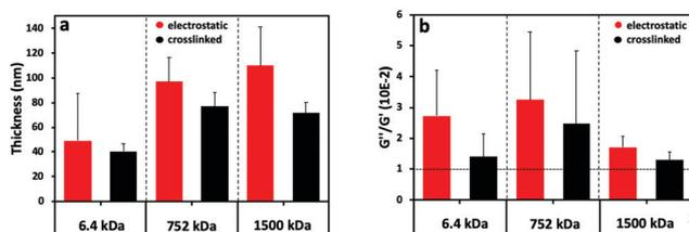
Fig. 2 (a) Hydrodynamic film thickness obtained by fitting the QCM-D data (5th, 7th and 9th overtones) according to the Voigt model and (b) viscoelastic properties shown by the ratio  $G''/G'$  of the (PLL-HA)<sub>5</sub> assemblies prepared with HA of different  $M_w$ s.
