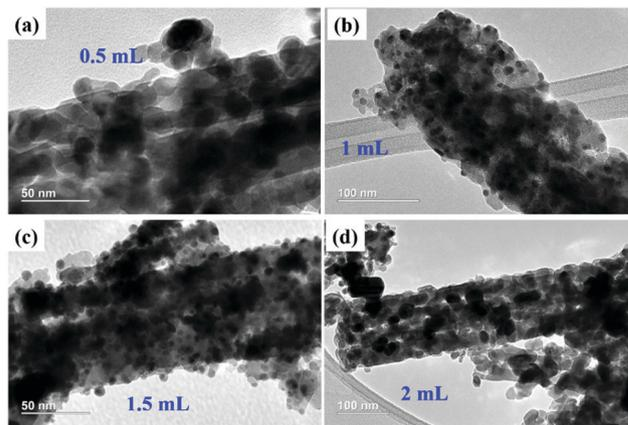
Fig. 6 TEM images of (a) 0.5-Au/Co<sub>3</sub>O<sub>4</sub> NRs, (b) 1-Au/Co<sub>3</sub>O<sub>4</sub> NRs, (c) 1.5-Au/Co<sub>3</sub>O<sub>4</sub> NRs, and (d) 2-Au/Co<sub>3</sub>O<sub>4</sub> NRs.
