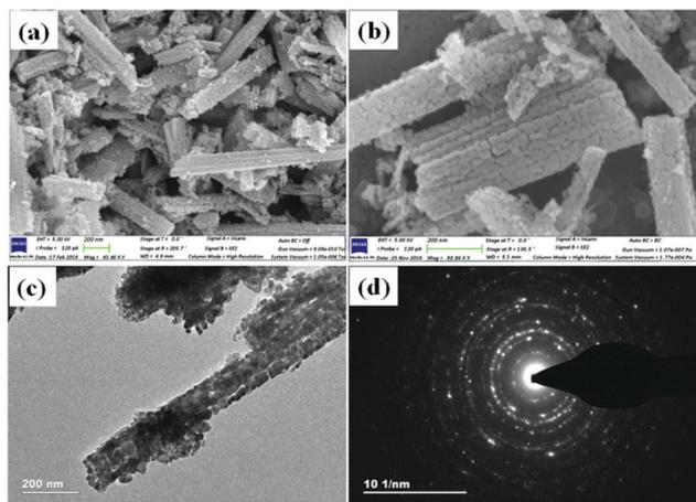
Fig. 3 FESEM of  $\text{Co}_3\text{O}_4$  NRs at (a) 43 K $\times$  magnification and (b) 88 K $\times$  magnification highlighting the pores and TEM (c) images (prepared as per the synthesis process in the Experimental section); (d) selected area diffraction (SAED) pattern of polycrystalline  $\text{Co}_3\text{O}_4$  structures.
