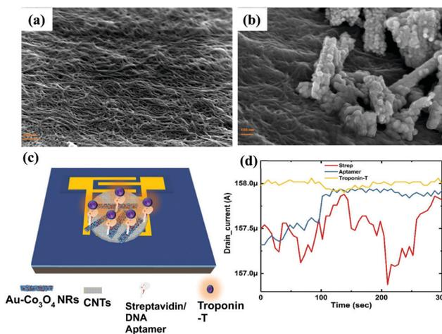
Fig. 7 SEM image of (a) SWCNTs on the Si/SiO<sub>2</sub> substrate, (b) Au/Co<sub>3</sub>O<sub>4</sub> NRs on top of the SWCNTs, (c) the FET with immobilized bilayer-2, and (d) the transient response (drain current) of the CNT device alone at multiple stages of functionalization.
