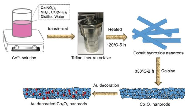
Fig. 1 Schematic illustration of the synthesis process of Co<sub>3</sub>O<sub>4</sub> and Au-decorated Co<sub>3</sub>O<sub>4</sub> NRs with the hydrothermal method using an autoclave and calcination approaches.
