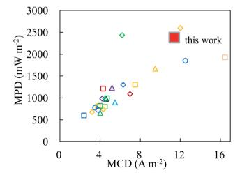
Fig. 7 (d) Comparison of the Fe-clusters/NAC catalysts with other Fe/NC catalysts reported in the last five years (MPD = maximum power density, MCD = max current density, see details in Table S3).
