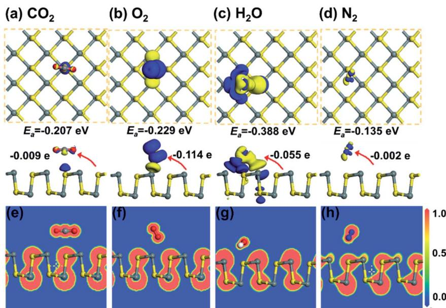
Fig. 4 The CDD for (a) CO<sub>2</sub>, (b) O<sub>2</sub>, (c) H<sub>2</sub>O, and (d) N<sub>2</sub> adsorbed on monolayer SnS. The isosurface is taken as 0.003 e Å<sup>-3</sup>. (e)–(h) show the corresponding ELF plots. Reprinted with permission from ref. 71. Copyright 2019, © IOP Publishing. All rights reserved.
