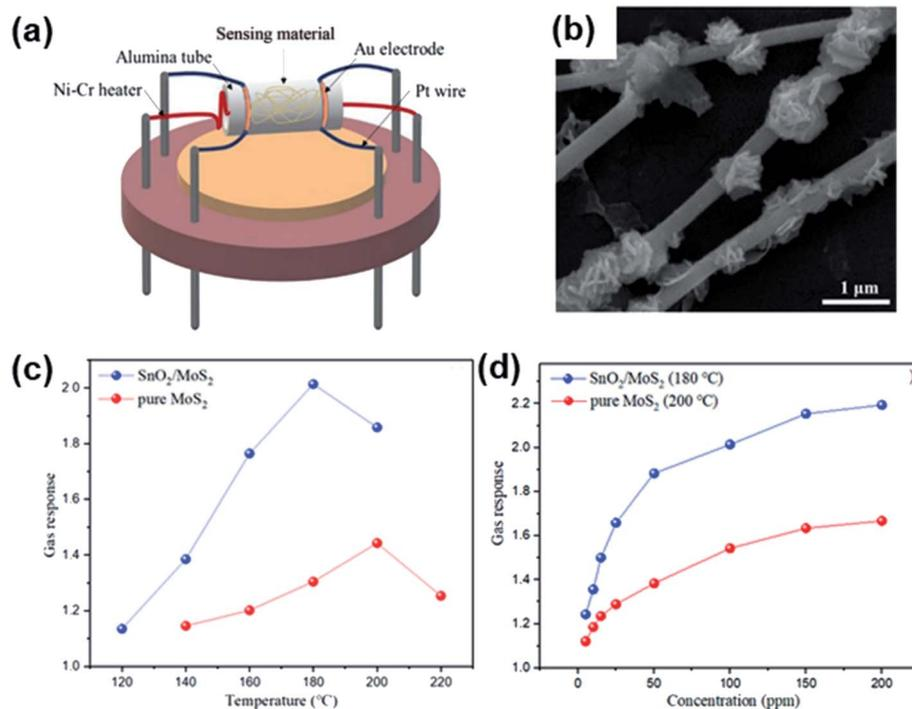
Fig. 20 (a) Schematic structure of a SnO<sub>2</sub>/MoS<sub>2</sub> gas sensor. (b) SEM results of SnO<sub>2</sub>/MoS<sub>2</sub> samples. (c) Gas response of sensor devices to 100 ppm CH<sub>4</sub> under different operating temperatures. (d) Gas response of two sensors to CH<sub>4</sub> with various concentrations. Reprinted with permission from ref. 163. Copyright 2019, Elsevier.
