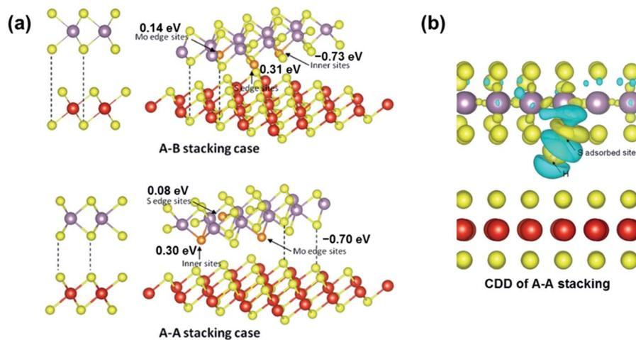
Fig. 12 (a) Two types of stacked bilayer structural models and their adsorption configurations. (b) CDD of the A-A stacking case (right) of the  $\text{VS}_2@MoS_2$ -edge nanosheet. The cyan and yellow regions represent the charge depletion and accumulation space, respectively. Reprinted with permission from ref. 35 Copyright 2017, ACS Publishing.
