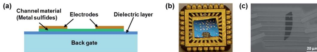
Fig. 17 (a) Schematic of an FET gas sensor. (b) Optical image of the MoS<sub>2</sub> transistor sensor on a chip. (c) SEM image of a two-layer MoS<sub>2</sub> transistor. Reprinted with permission from ref. 83. Copyright 2013, ACS Publishing.
