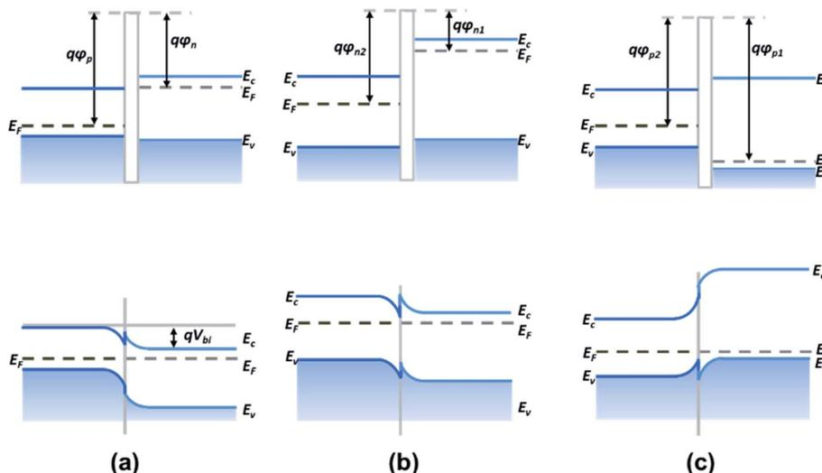
Fig. 16 Band alignment of (a) p–n junctions, (b) n–n junctions, and (c) p–p junctions.  $E_c$ ,  $E_f$ , and  $E_v$  are the conduction band edge, Fermi level, and valence band edge of the semiconductor, respectively.  $\phi_p$ ,  $\phi_n$ , and  $V_{bi}$  are the p-type semiconductor work function, the n-type semiconductor work function, and the built-in potential barrier, respectively.<sup>116</sup>
