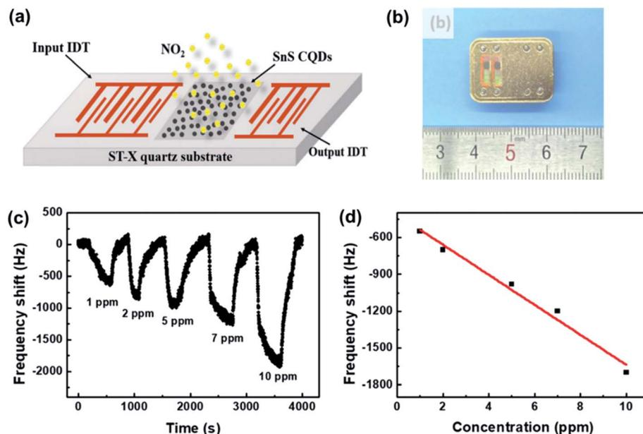
Fig. 19 (a) The schematic and (b) a photograph of the SAW sensor based on SnS CQDs. (c) The response curves of the SAW sensor to different  $\text{NO}_2$  concentrations. (d) The dependence of the response on  $\text{NO}_2$  concentration. Reprinted with permission from ref. 140. Copyright 2019, Elsevier.
