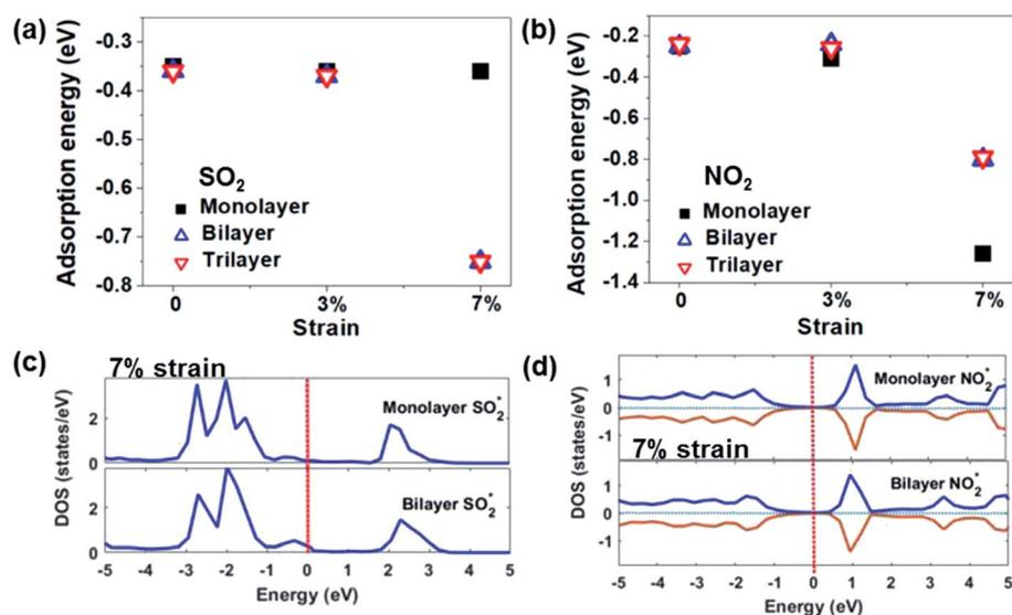
Fig. 8 Adsorption energies of (a) SO<sub>2</sub> and (b) NO<sub>2</sub> on 1T'-MoS<sub>2</sub> sheets with a different number of layers and different strains. Total DOS of MoS<sub>2</sub> monolayer and bilayer systems at 7% strain adsorbed by (c) SO<sub>2</sub> and (d) NO<sub>2</sub>. Reprinted with permission from ref. 79. Copyright 2019, ACS Publishing.
