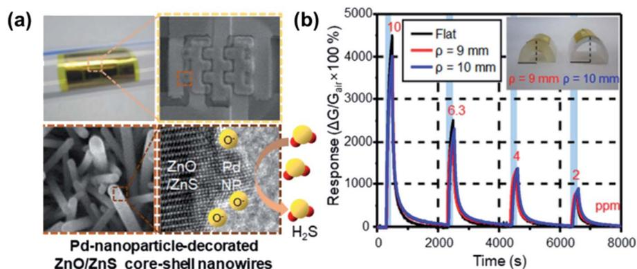
Fig. 29 (a) Photograph and SEM and TEM images of a ZnO/ZnS NW sensor on a flexible substrate and (b) the H<sub>2</sub>S gas sensing result. Reprinted with permission from ref. 132. Copyright 2019, ACS Publishing.
