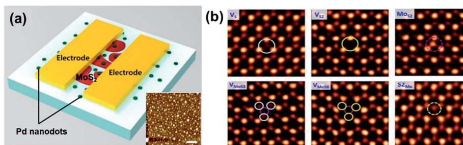
Fig. 14 (a) Schematic of a Pd-doped MoS<sub>2</sub>-based sensor. The inset image shows the AFM image of Pd on a SiO<sub>2</sub> substrate. The scale bars indicate a distance of 400 nm. Reprinted with permission from ref. 107. Copyright 2017, Elsevier. (b) Image analysis for intrinsic point defects in ML MoS<sub>2</sub>. Reprinted with permission from ref. 36. Copyright 2013, ACS Publishing.
