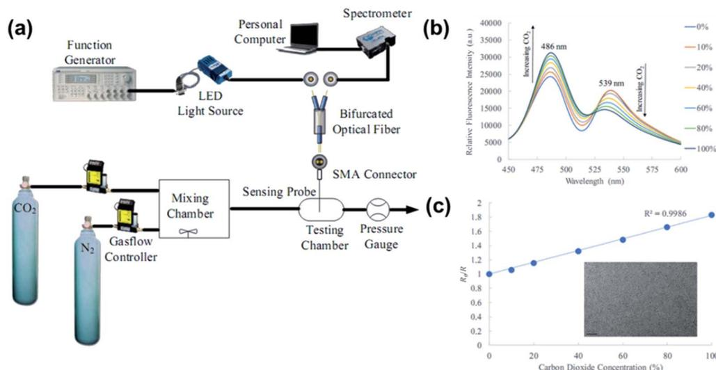
Fig. 28 (a) Experimental setup for the ratiometric optical fibre CO<sub>2</sub> sensing. (b) Fluorescence spectra of the ratiometric optical fibre sensor under different CO<sub>2</sub> concentrations. (c) Calibration curve of the ratiometric optical fibre CO<sub>2</sub> sensor at 0–100% concentration. Reprinted with permission from ref. 225. Copyright 2019, SPIE publishing.
