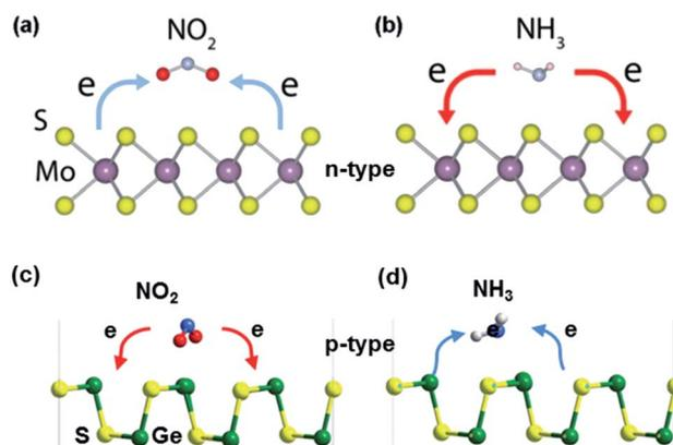
Fig. 6 Gas sensing mechanism of (a and b) MoS<sub>2</sub> (n-type metal sulfide). Reprinted with permission from ref. 27. Copyright 2018, ACS Publishing. (c and d) GeS (p-type metal sulfide) in the presence of NO<sub>2</sub> and NH<sub>3</sub> molecules. Reprinted with permission from ref. 77. Copyright 2018, The Royal Society of Chemistry.
