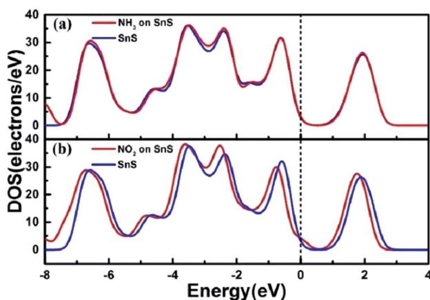
Fig. 5 The total DOS for (a) NH<sub>3</sub> and (b) NO<sub>2</sub> adsorbed on monolayer SnS. The Fermi level is set as zero. Reprinted with permission from ref. 72. Copyright 2017, IEEE.
