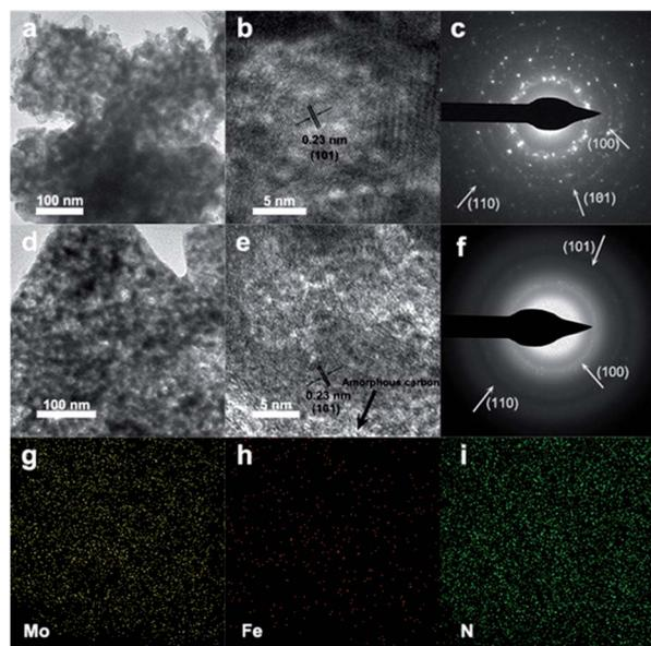
Fig. 2 (a) TEM image, (b) HRTEM image, and (c) SAED pattern of pure  $\beta$ -Mo<sub>2</sub>C. (d) TEM image, (e) HRTEM image, and (f) SAED pattern of 0.5% Fe-Mo<sub>2</sub>C@NCF. The corresponding EDS mapping images of (g) Mo, (h) Fe and (i) N for 0.5% Fe-Mo<sub>2</sub>C@NCF.
