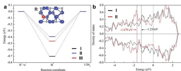
Fig. 6 (a) Free energy diagrams of the HER on pristine Mo<sub>2</sub>C (I), 0.5% Fe-Mo<sub>2</sub>C (II) and 1% Fe-Mo<sub>2</sub>C (III). (b) Partial density of states of the Mo-3d states at the adsorption sites on pristine Mo<sub>2</sub>C (I) and 0.5% Fe-Mo<sub>2</sub>C (II). The d-band center of each material is labelled with corresponding values.
