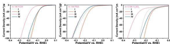
Fig. 5 The iR-corrected polarization curves at a scan rate of 5 mV s<sup>-1</sup> of (I) 0.5% Mn-Mo<sub>2</sub>C@NCF, (II) 0.5% Fe-Mo<sub>2</sub>C@NCF, (III) 0.5% Co-Mo<sub>2</sub>C@NCF, and (IV) 0.5% Ni-Mo<sub>2</sub>C@NCF electrocatalysts in 1.0 M KOH (a), 1.0 M PBS (b), and 0.5 M H<sub>2</sub>SO<sub>4</sub> (c).
