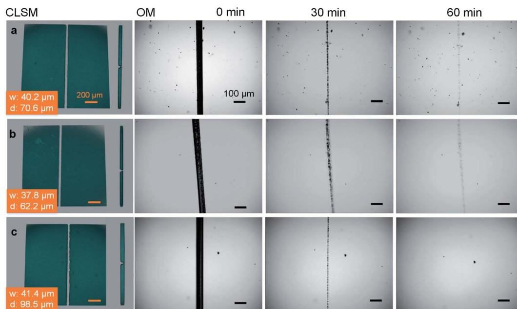
Fig. 1 Self-healing of 30PHS/PEOZ with  $\text{CaCl}_2$ . 3D laser microscopic images and optical photographs of the self-healing process of (a) 30PHS/PEOZ, 30PHS/PEOZ with (b) 0.17 equivalent  $\text{CaCl}_2$  and (c) 0.25 equivalent of  $\text{CaCl}_2$ . The healing rate of 30PHS/PEOZ was improved by the addition of 0.25 equivalent of  $\text{CaCl}_2$ . CLSM: confocal laser scanning microscope, OM: optical microscope, w: width, d: depth.
